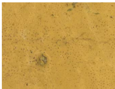
Fig. 2: Pinholes in a film due to solvent entrapment
