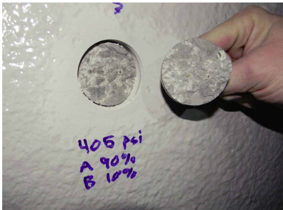
Fig. 9: Pull-off adhesion testing. 90% of the failure occurred cohesively within the substrate, whereas 10% of the failure occurred cohesively within the filler/surfacer.
