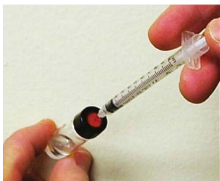
Fig. 5: Transferring blister liquid from syringe to a glass septum vial
