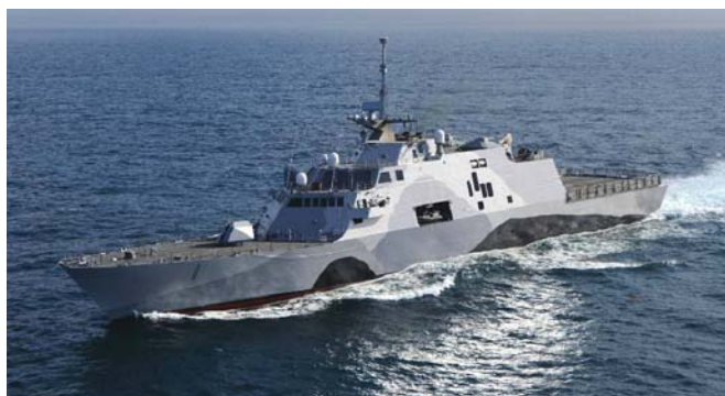
The four-color camouflage pattern on the USS Freedom was applied with a color-stable, low solar-absorbing, low-VOC coating system. Photo courtesy of David Clapp.
