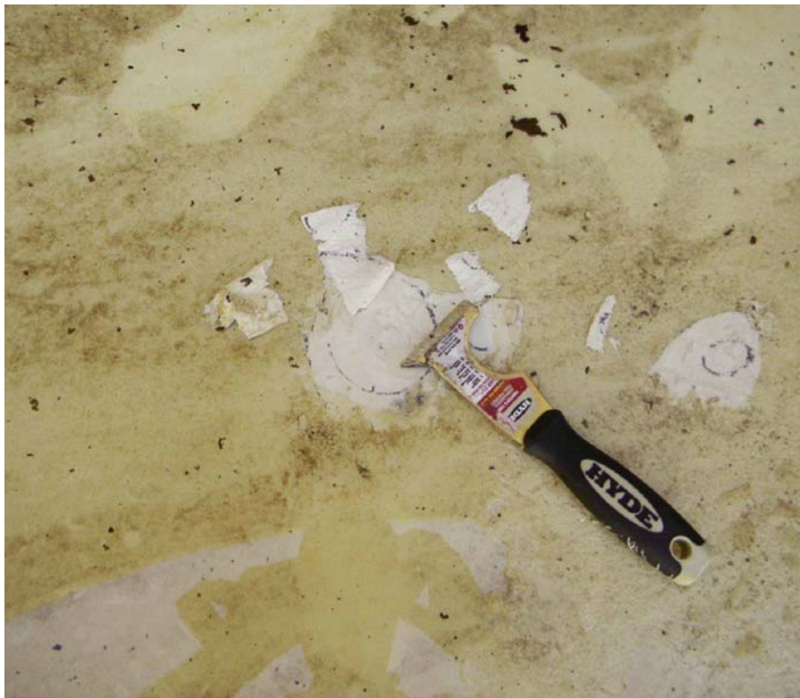
Fig. 12: Off-ratio repair material found during anniversary inspection
