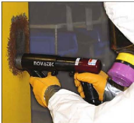
A needle scaler is a reciprocating impact tool that works well on vertical as well as irregular surfaces. Courtesy of Novatek Corp.
