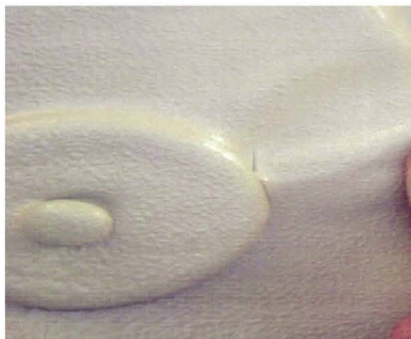
Fig. 6: Void at edge of mechanical anchor
