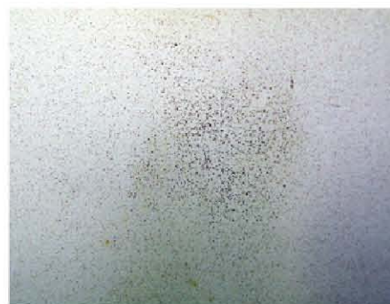
Fig. 2: Pinpoint rusting through the topcoat
