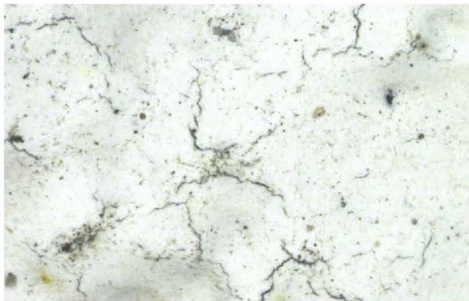
Fig. 5: Stress fracturing or cracking caused by excessive film thickness, viewed at 50x
