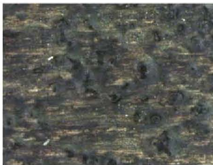
Fig. 9: Blisters in a clear coat applied at three times the recommended thickness over wood substrate
