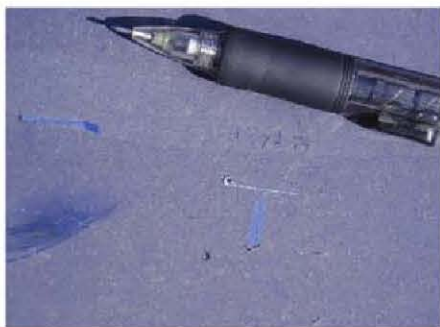
Fig. 8: Washed coated surface. Dirt is embedded into the top coating layer.
