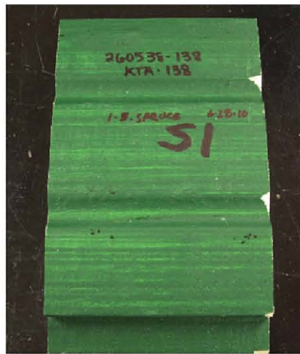
Fig. 1: Scant coating coverage of wood siding. The substrate is visible through the thin coating material. Figures courtesy of the author.
