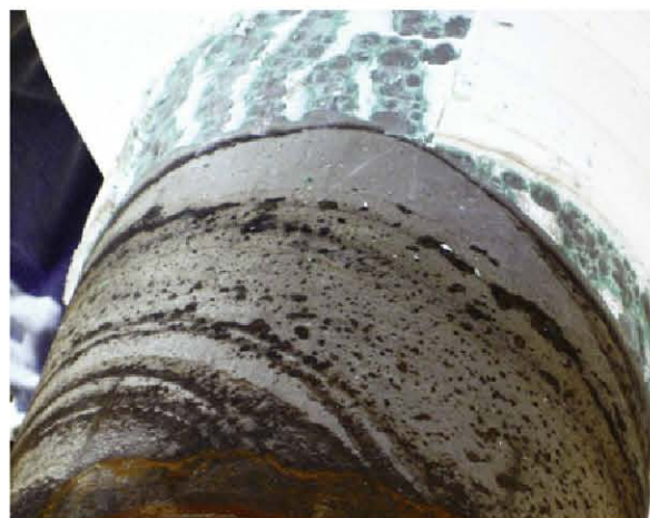
Fig. 5: For larger disbondments, there are often growth rings with alternating cathodic and anodic areas. This suggests that wet and dry cycles play a part in the rate of disbondment.
