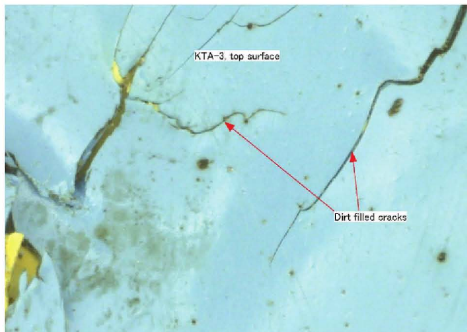
Fig. 3: Cracked topcoat of a system applied approximately 20 mils below the minimum specified thickness range, viewed at 50x
