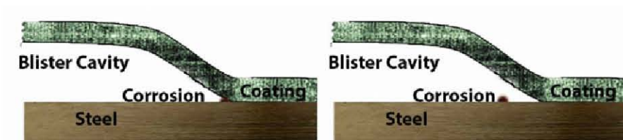
Fig. 6: Illustration of anodic delamination scenario on the left; cathodic on right. 3
