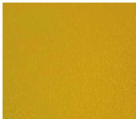
Fig. 7: Wrinkles caused by a coating applied at four times the recommended thickness
