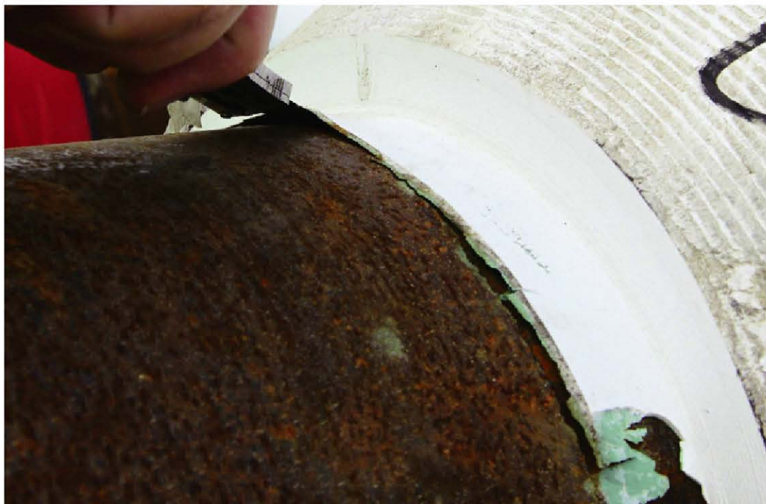
Fig. 1: Occasionally, for multi-layer polyolefin systems, the FBE disbands from the steel in the girth weld area.
