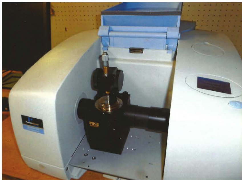
Fig. 3: Pictured is a Fourier transform infrared spectrometer, displaying an attenuated total reflectance (ATR) accessory mounted in the sample compartment. ATR allows spectra to be obtained from surfaces of very small samples.
