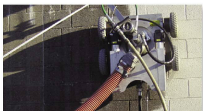
SRT-10 Crawler Work high with no fall risk; wireless controls
