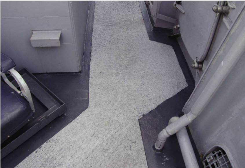
Fig. 3: This photo shows a qualified MIL-PRF-24667C, Type I epoxy non-skid that has become white due to blooming.
