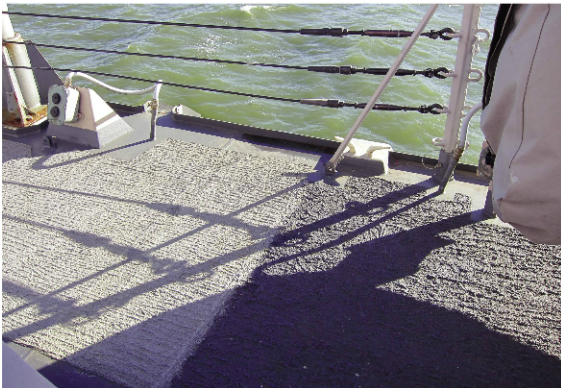
Fig 4: This picture depicts a qualified Type V epoxy non-skid (left) compared to the siloxane non-skid (right) after six months of exterior exposure on the USS MASON (DDG-87).
