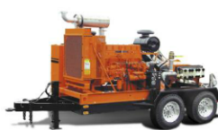
NLB Pump Unit Easily converts to 8 pressures, up to 40,000 psi; 1,000 hp max.
