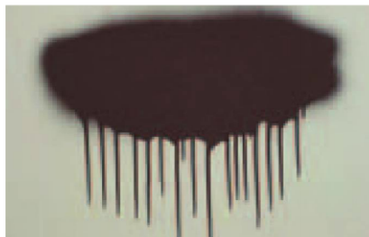
The photo at left shows satisfactory drip from a new spray tip, while the photo at right shows a drip pattern indicating that the spray tip is worn.
