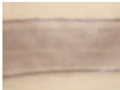
The tail pattern in this photo is a result of too little application pressure.
