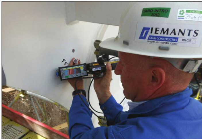
Van Poppel performs pull-off adhesion testing during the Stinger pipeline installation project in Vlissingen, the Netherlands. This large oil and gas pipeline was mounted on a vessel, which supports pipe sections of up to 68 feet, in very deep ocean water. Photo courtesy of Ronny Van Poppel.
