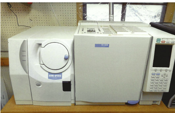
Fig. 2: A GCMS. The module to the left is the mass spectrometer, and the module to the right is the actual gas chromatograph (most of which is comprised of the oven).
