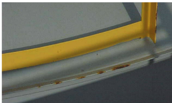
Edge failure evident on yellow angle
