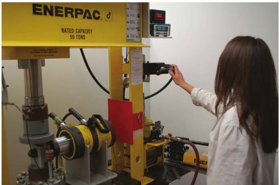
Fig. 8: Electronic displays of clamping force and slip deflection
