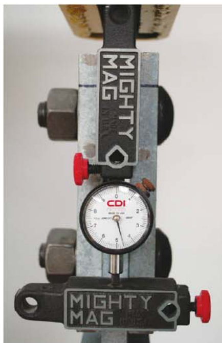
(top left) Fig. 10: Illustration from Appendix A of the RCSC specification showing the tension creep chain assembly (above right) Tension creep test in progress (bottom left) Close-up of micrometer and magnets attached to assembly
