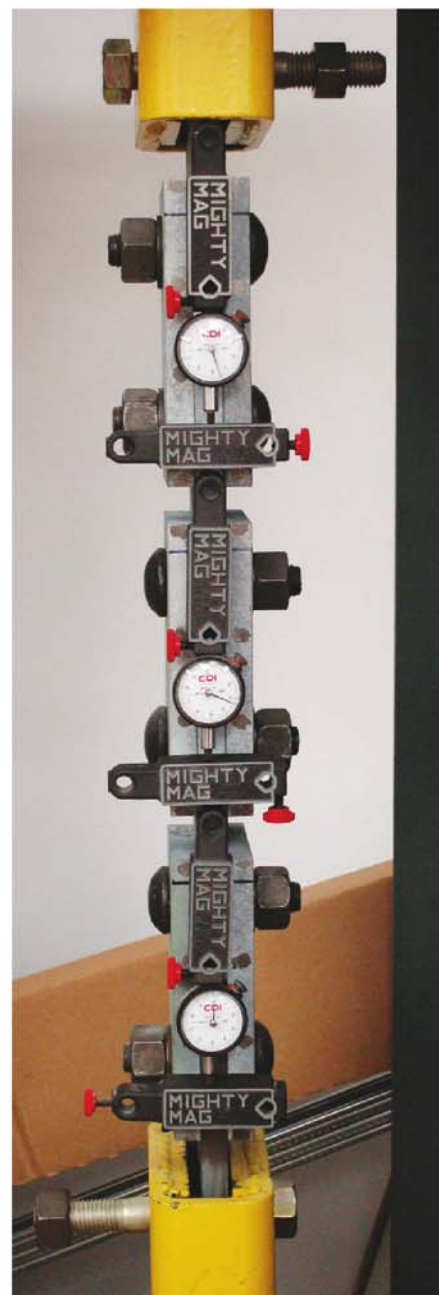
(top left) Fig. 10: Illustration from Appendix A of the RCSC specification showing the tension creep chain assembly (above right) Tension creep test in progress (bottom left) Close-up of micrometer and magnets attached to assembly
