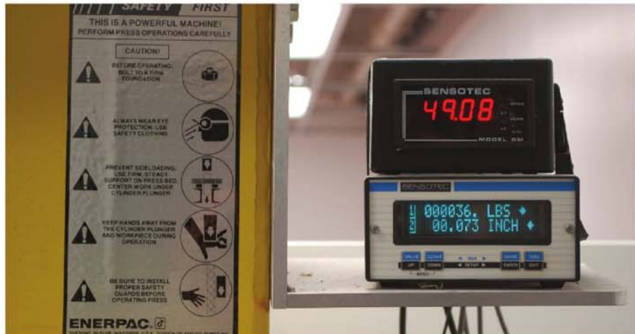
Fig. 8: Electronic displays of clamping force and slip deflection
