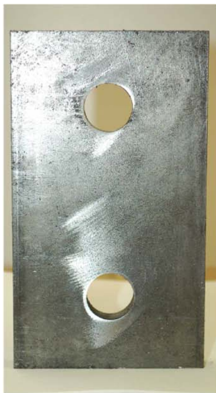
(left) Fig. 1: Slip Test Plate (front view). The hole has been deburred. (bottom) Fig. 2: Slip Test Plate (end view). The edge has been milled flat. (right) Fig. 3: Tension Creep Test Plate (front view). The holes have been deburred.
