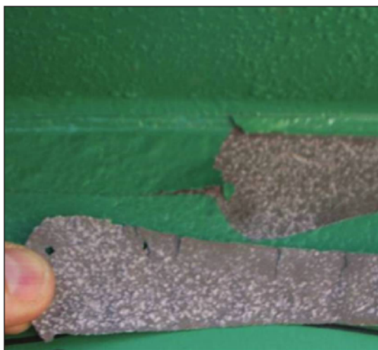
Fig. 6: Close-up of zinc salt formation on the zinc-rich primer surface, beneath the removed blistered finish coat
