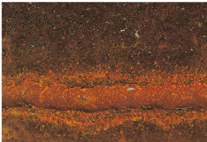
Fig. 1: (Left) Unpainted steel, pitted and rusted. (Right) The same steel specimen after hand tool cleaning to SSPC-SP 2. Courtesy of SSPC. Note: Fig. 1 and Fig. 2 are not equal in photographic quality to the actual reference photographs in VIS 3 and should not be used as substitutes for the actual standard.
