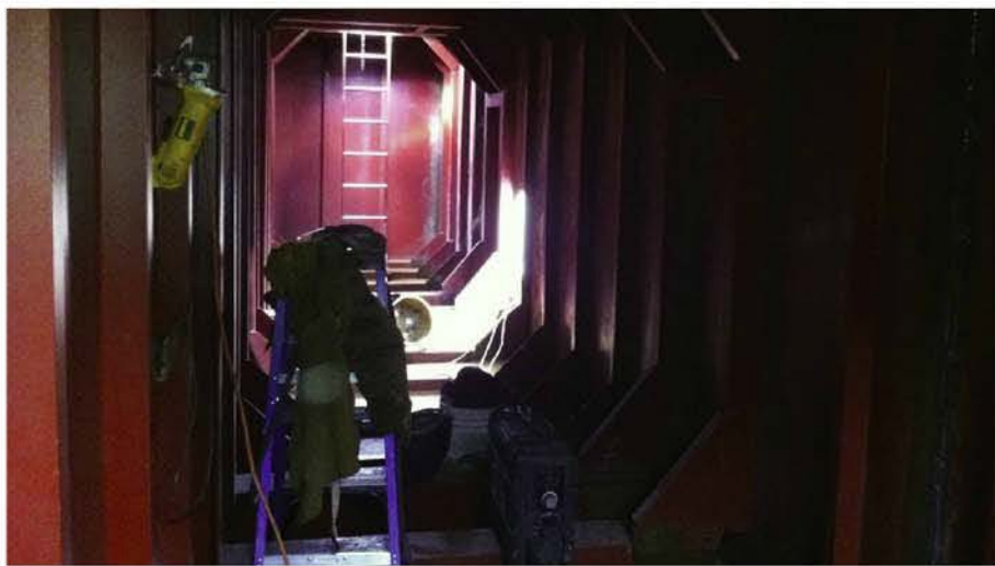
This interior of a ballast tank on a barge is a PRCS.
