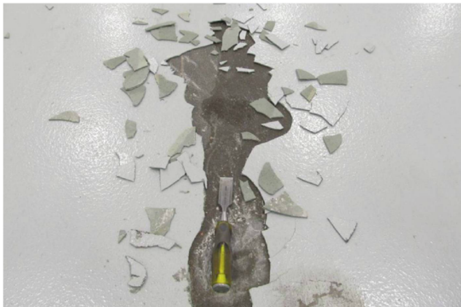
Fig. 4: Running a chisel against an exposed edge caused cracking and delamination of the coating.
