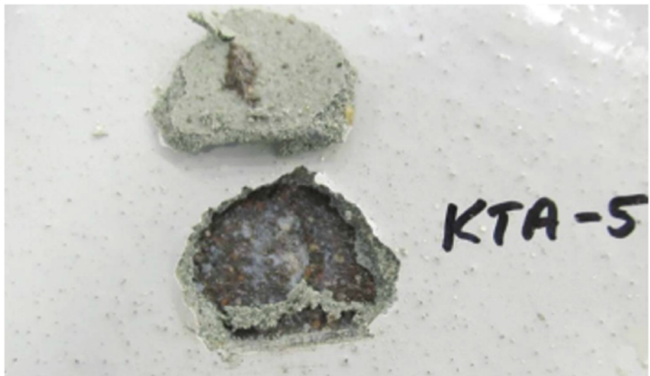
Fig. 3: An opened blister shows the plane of separation between base and cap.
