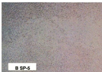
Fig. 2: Samples of degrees of blast cleaning on steel covered with rust and millscale, from SSPC's VIS-1, Guide and Reference Photographs for Steel Surfaces Prepared by Dry Abrasive Blast Cleaning. Courtesy of SSPC. Not to be used in place of the actual visual standard.
