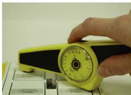
Fig. 4: (top) and 5 (bottom) Verifying the accuracy of Type 1 gages using certified coated thickness standards
