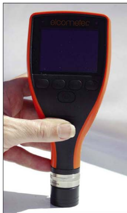
Fig. 3: Example of electronic DFT gage categorized as Type 2 in SSPC-PA 2
