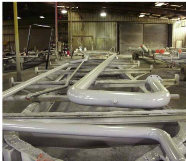
Fig. 15: (top and left): Appendix 7 of the 2012 edition of SSPC-PA 2 describes a method for measuring DFT on non-flat steel, such as pipe sections that can be loaded on racks or carts. Photos courtesy of Turner Industries Group, L.L.C.
