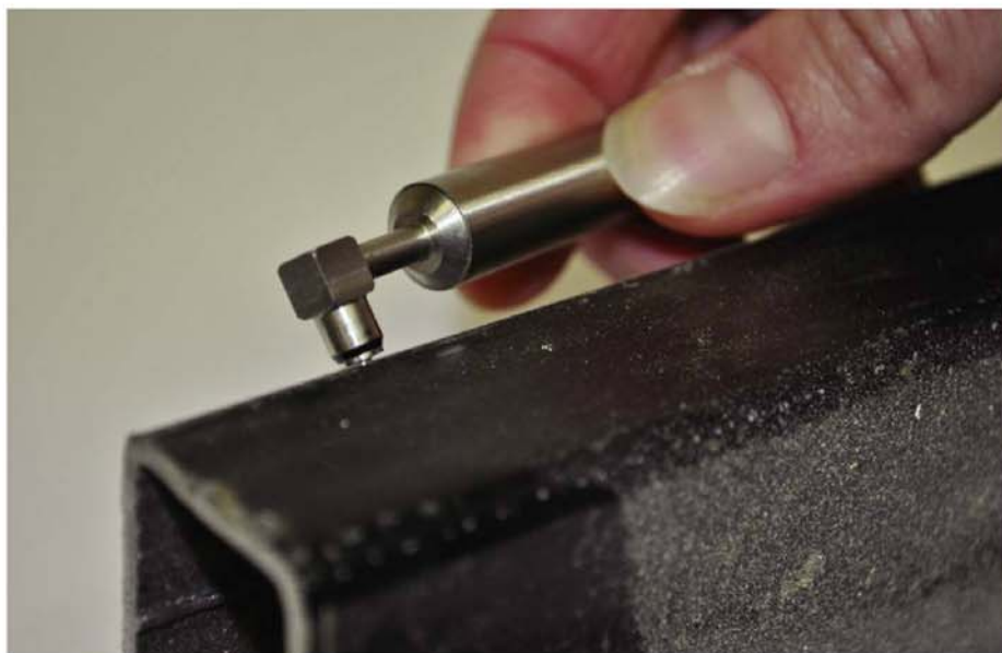
Fig. 14: One of a variety of Type 2 gage probe configurations designed to better measure DFT of coatings on edges
