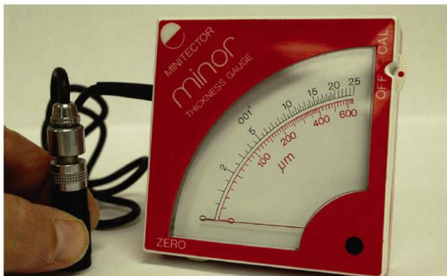
Fig. 1: One type of magnetic gage referenced in original SSPC-PA 2 for measuring dft Figures courtesy of the author except where otherwise indicated
