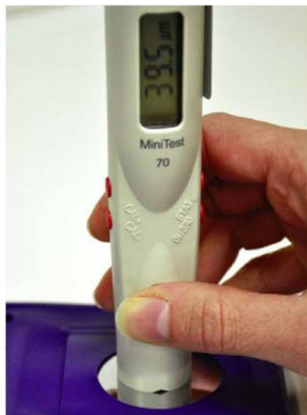
Fig. 7: Verifying accuracy of Type 2 gage on a certified coated standard
