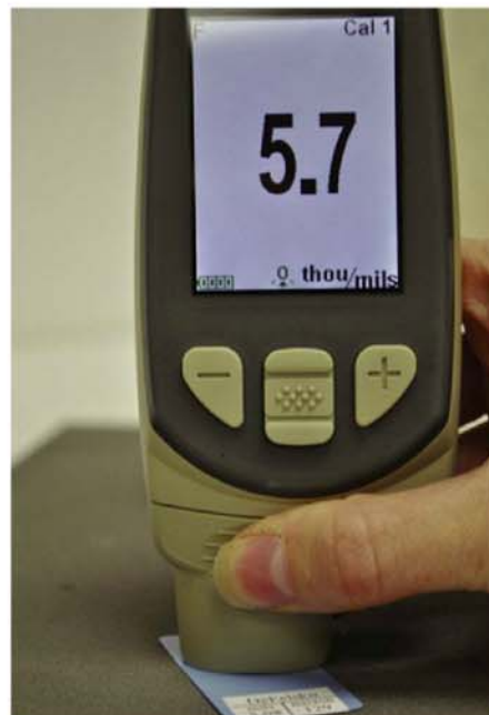
Fig. 9: Adjusting Type 2 gage using a measured shim on the surface to which the coating will be applied
