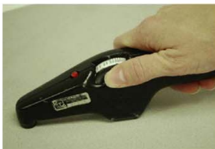
Fig. 6: Obtaining base metal readings with Type 1 gage
