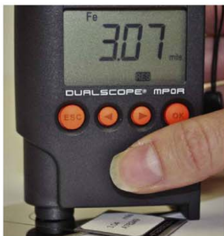
Fig. 8: Verifying accuracy of Type 2 gage using a certified shim
