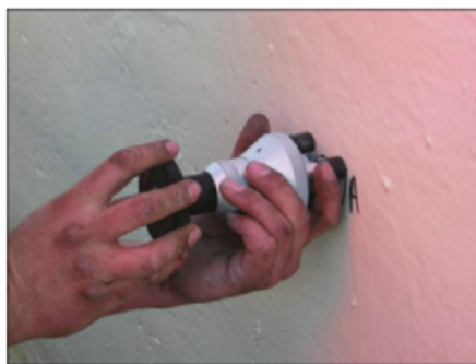
Fig. 5: Type II gauge has a maximum pull-off adhesion limit of 1,000 psi.
