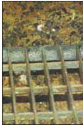
Fig. 2: HCl acid attack in petrochemical plant
