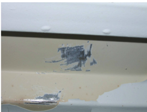
Fig. 3: Adhesion of the original alkyd to the steel was excellent. Aggressive scraping was needed to remove the alkyd.
