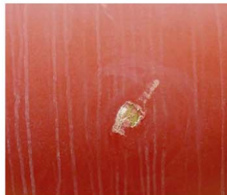
Fig. 6: Minor mechanical defect observed on the pipe body.
