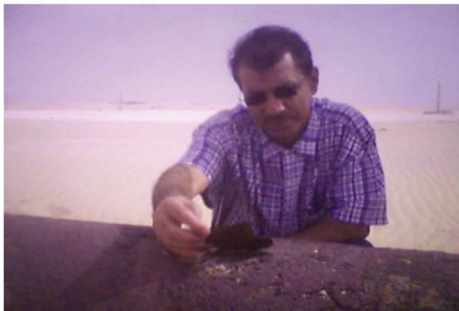
Fig. 2: Examination of corrosion deposit scale on failed old tape wrap pipeline removed from service
