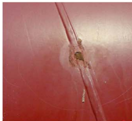
Fig. 5: 46-inch Ø Pipe FBE damage on spiral girthweld
