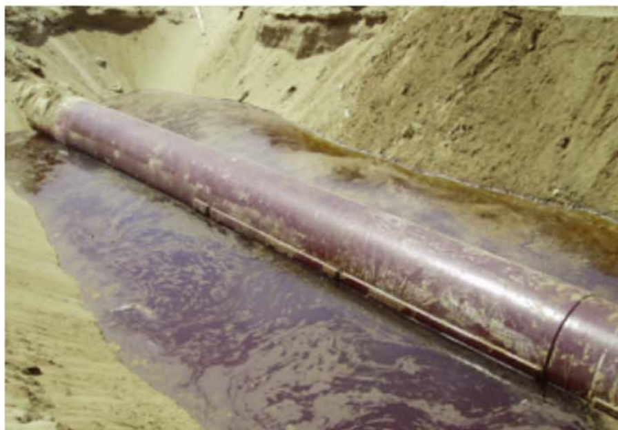
Fig. 4: Buried FBE pipe in Sabkha wet sand bordered with water had deficiencies within five years in service.
