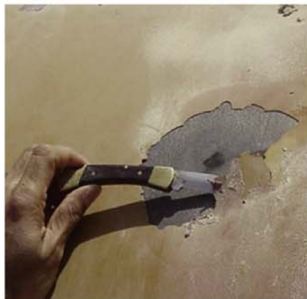
Fig. 10: Unidentified black spots under damaged coating were observed at the 11 o'clock position.
