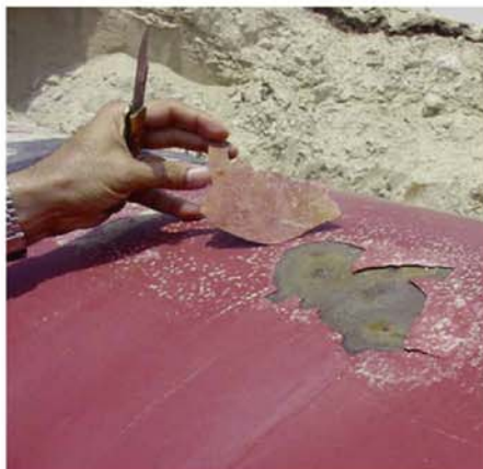
Fig. 11: FBE delamination at the 12 o'clock position was caused by mechanical damage.
