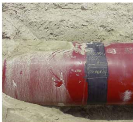
Fig. 8: The heat shrink sleeve for girthweld pipe joint protection was found in satisfactory condition in dry sand only.
