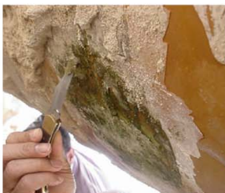
Fig. 13: Poor repair workmanship at girth weld using liquid epoxy coating at the 6 o'clock position.
