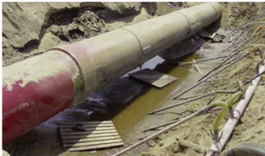
Fig. 9: The FBE in wet Sabkha found with blisters and corrosion under the FBE coatings.
