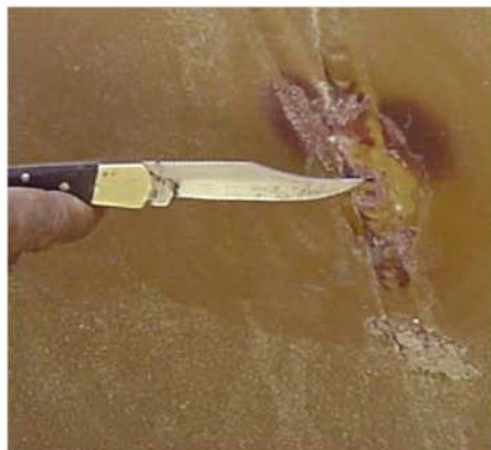
Fig. 7: Defects at repaired girth weld area at the 7 o'clock position due to incomplete weld beads.
