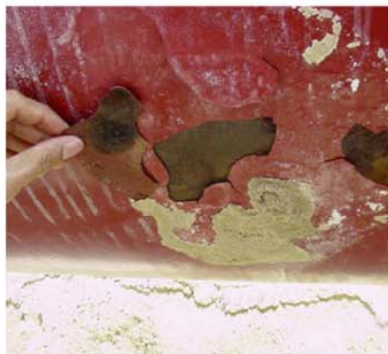
Fig. 12: FBE coating blisters at 5 o'clock position in wet Sabkha area, which was exposed to the water table.
