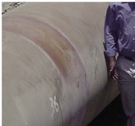
Fig. 14: The FBE color discoloration and fading, which is common with epoxy coatings
