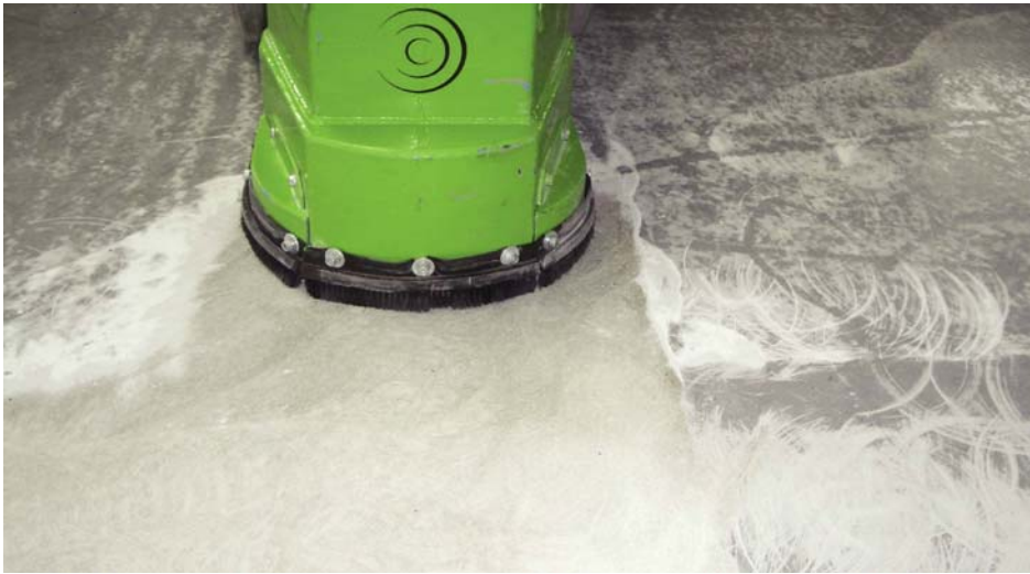
Fig. 4: Paint removal by a single-head, three-phase grinding machine
