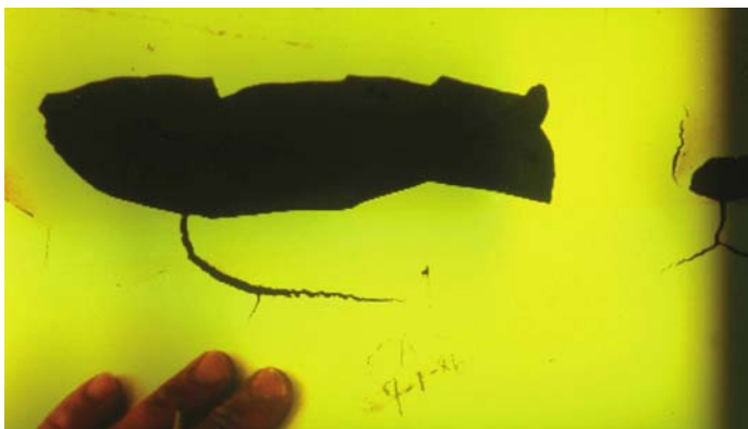
Fig. 4: Spontaneous cracking of the coating along the fillet weld
