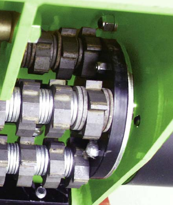
Fig. 1: (Above): Underside of small planing machine showing milling flail drum Photos courtesy of the author
