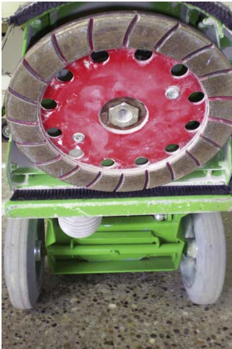
Fig. 5: Underside of grinding machine showing diamond plate
