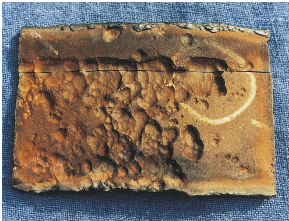
Fig. 4: Microbiologically influenced corrosion on piece of steel pipe Courtesy of the author
