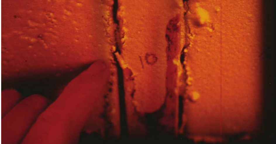
Fig. 8: Area where epoxy mastic was applied directly to the steel rather than the aged alkyd
