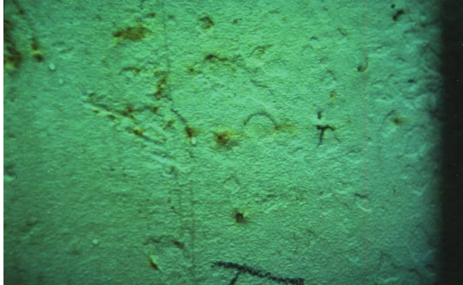
Fig. 6: Corrosion of steel beneath alkyd primer evident within six months
