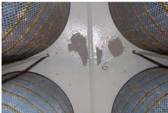
Fig. 3: Delamination of the topcoat often occurred between the filters
