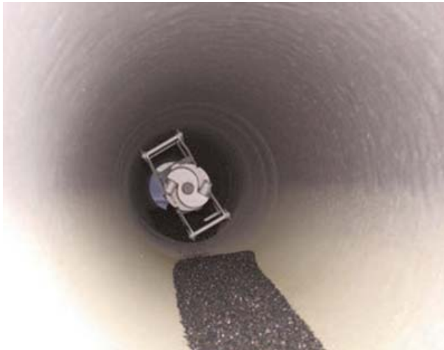
Fig. 6: Rotary abrasive blasting the interior surfaces of ductile iron pipe
