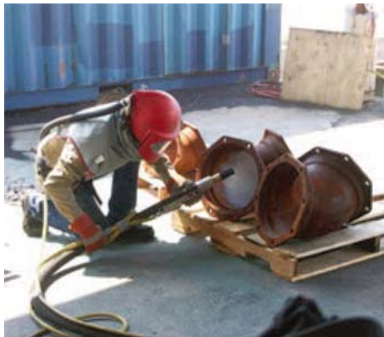
Fig. 7: Uniformly abrasive blasting the interior surfaces of cast iron fittings using an angular abrasive
