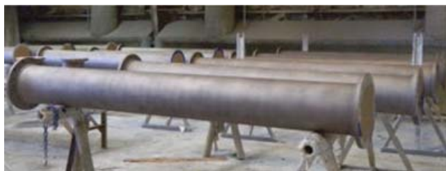
Fig. 5: Ductile iron pipe exterior prepared in accordance with NAPF 500-03-04 External Pipe Surface
