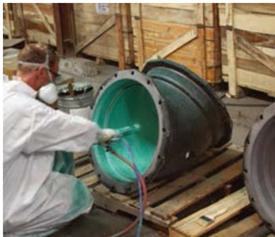
Fig. 8: Internally lining a ductile iron fitting following a Blast Clean#1 condition, 3.0 mils anchor profile
