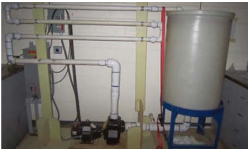
Fig. 3: High flow water test set up. Samples were placed inside 1.5-inch PVC pipe.
