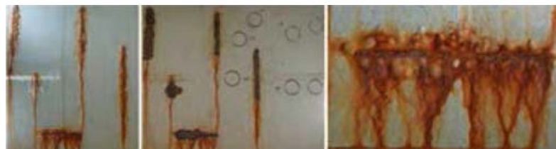
Fig. 7: Photographs of test panels S2T3 (DHP4) after six months of C5M test – (left): before coating removal around the scribe, (center): details of scribe 3 and (right): after coating removal.
