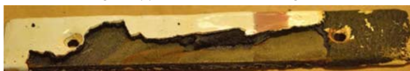
Fig. 5: Failure of overcoated coal tar during a high flow test
