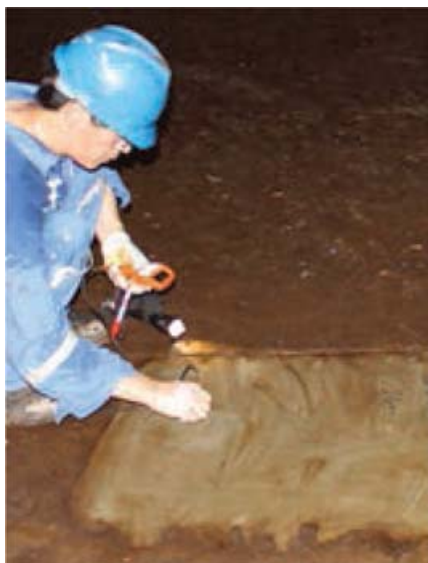
Fig. 3: Abrasion-resistant, aluminum pure epoxy coating "after 15 years in service. Removal of the residual oil layer reveals the excellent condition of the coating and tank top beneath," according to the manufacturer.
