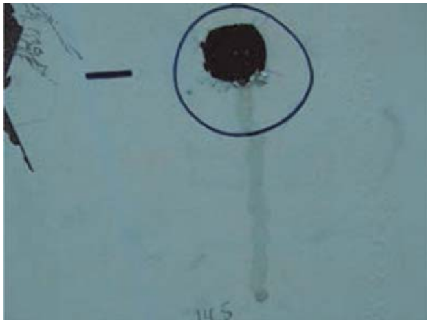
Fig. 2: After blisters were manually fractured, the underlying steel substrate showed a blackened appearance.
