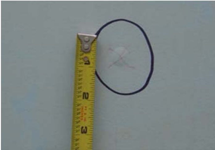
Fig. 1: Unbroken, liquid-filled blister. All photos courtesy of KTA-Tator, Inc.
