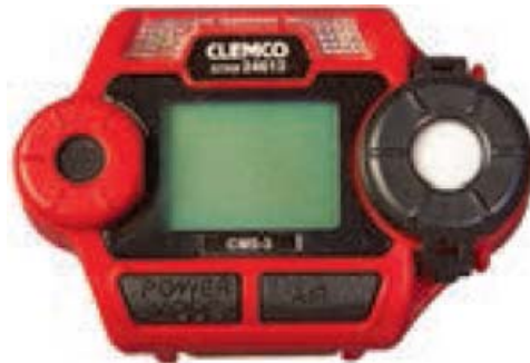
Fig. 4: CO monitor that may be used as an individual CO monitor
