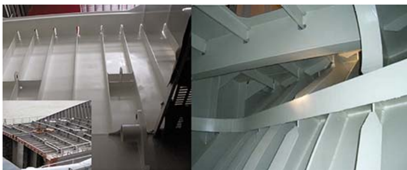
Edge profiles in maritime steel constructions From left: tank deck; offshore construction; cargo hold roof All photographs and drawings are courtesy of IFAM, Bremen; and Muehlhan AG, Hamburg.
