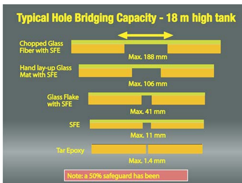
Fig. 2: Hole bridging capacity for different lining systems for an 18-meter (38-foot) high tank. (SFE: Solvent-free epoxy) 11
