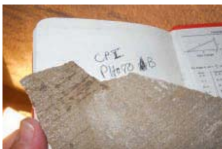
Fig. 6: Flexible polyurethane lining—cohesive failure within cementitious mortar—New Jersey
