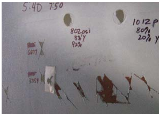
Fig. 1: An example of three adhesion tests conducted in close proximity to one another. Note that the tensile adhesion test resulted in values between 800 and around 1,000 psi—evaluated as acceptable. The knife adhesion test (ASTM D6677) and tape adhesion test (ASTM D3359) resulted in poor adhesion (0 and 2A, respectively).
