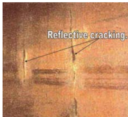
Fig. 10: Typical reflective cracking of an epoxy lining taken in sludge tank in Virginia in 1997. The lining was installed in 1992.
