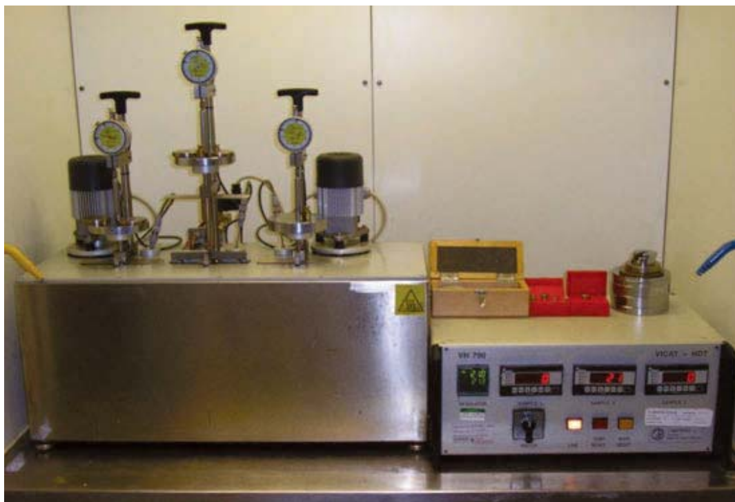
Fig. 3: VICAT heat distortion temperature equipment
