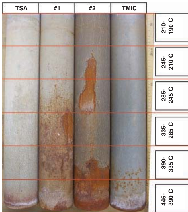
Fig. 7: After cyclic immersion in salt solution with dry out
