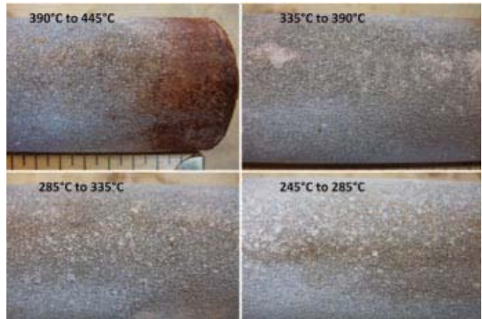
Fig. 11: TSA after CUI cyclic testing
