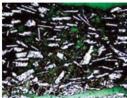
Fig. 26: SEM image of Coating #2 after image analysis to evaluate coating porosity after exposure at 400 C showing porosity level of 9% in the matrix (200 x)
