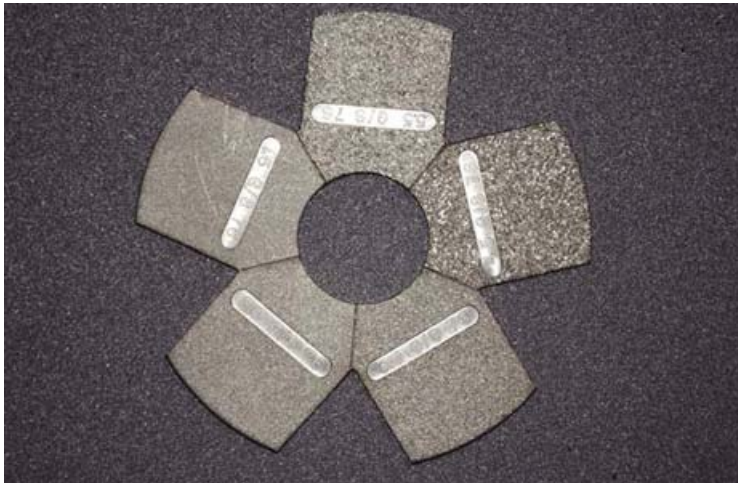
Fig. 7: Surface profile would be reported as 2 mils using the comparator (the surface closely matches the bottom left segment) and accepted as meeting a maximum 2-mil specification requirement. Photo courtesy of KTA
