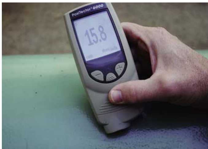
Fig. 6: A reading with a modern instrument on the same coating measured in Fig. 5 shows 15.8 mils. While the reading shown in
