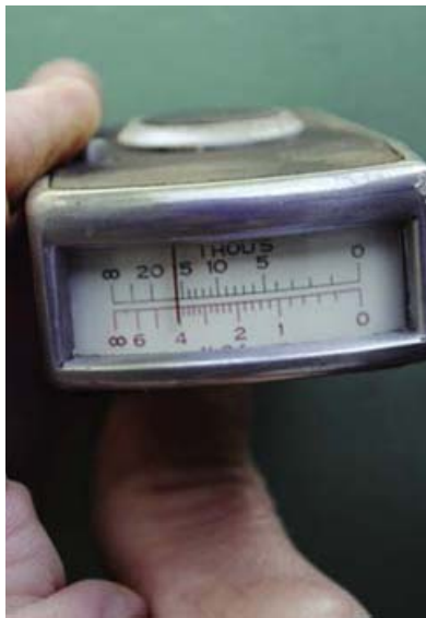
Fig. 5: The instrument used in 1966 shows a reading on a current pipe coating that would have been accepted as meeting a 16-mil minimum requirement. Photo courtesy of KTA
