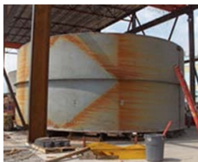
Fig. 1: Assembled stack section showing red rust staining pattern related to crating frames Photos courtesy of the author
