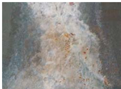
Fig. 4: White zinc corrosion products with spots of red rust occur where water stands on an IOZ-coated surface for extended periods.
