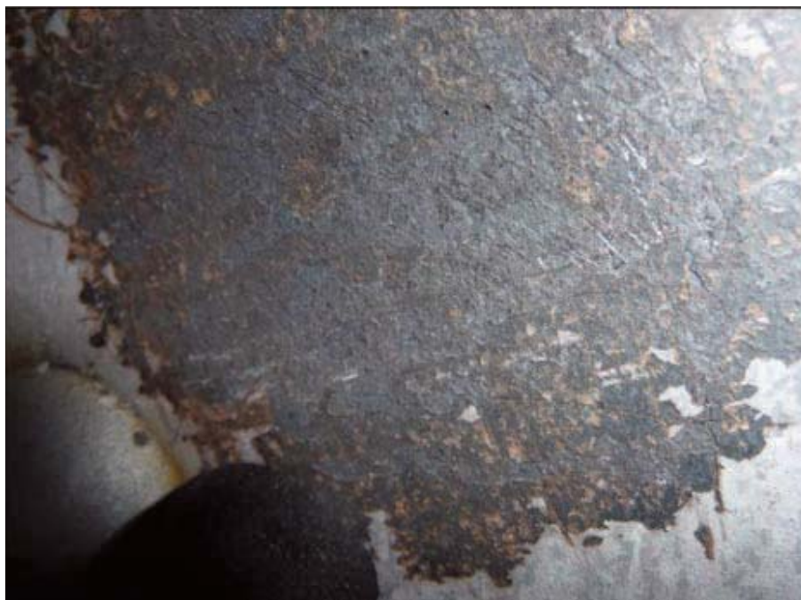
Fig. 4: The substrate beneath the new overcoat system contained a roughened mill scale surface.
