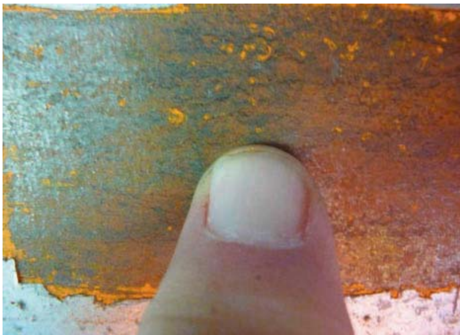
Fig. 1: Mill scale on the substrate beneath the lead-alkyd coating system. Photos courtesy of KTA-Tator, Inc.
