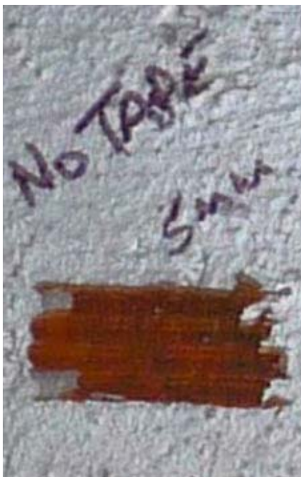
Fig. 6: An ASTM D3359 Method B (Cross-cut) Tape Test resulted in a 0B rating even before the tape could be applied.
