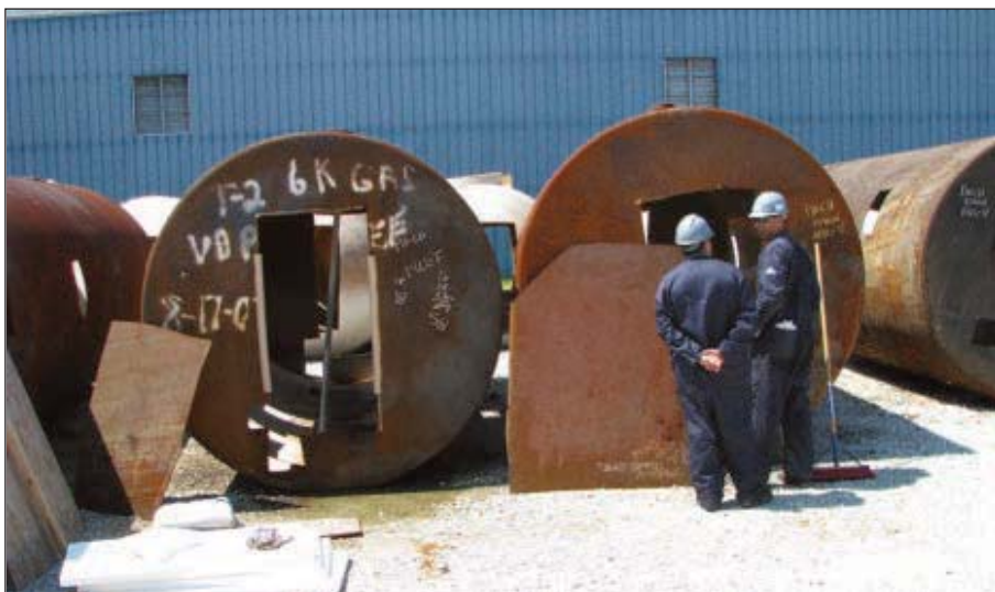
Fig. 1: Typical lined steel underground gasoline tanks removed from service stations and kept in a storage yard. Photos courtesy of KTA-Tator, Inc.
