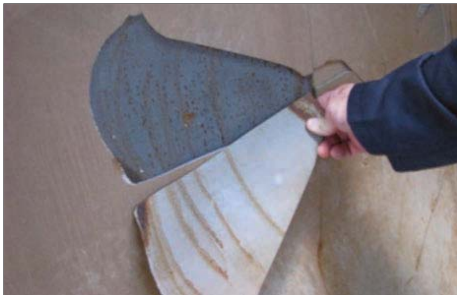
Fig. 3: Disbonding of epoxy lining from a steel tank interior. Note the blast cleaned steel beneath the delaminated epoxy lining.
