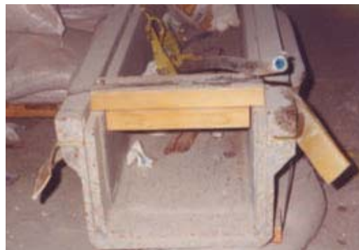
Portion of a pre-cast trench made of novolac epoxy polymer concrete, and the same epoxy novolac polymer was installed over the surrounding floors.
