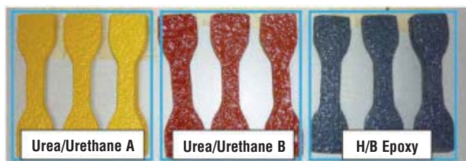
Fig. 2: Free film specimens for tensile strength test
