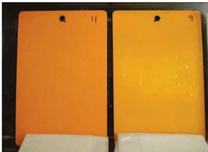
Fig. 2: Test panels for Systems #2 and #3 (comparable systems) showed no effect after moisture exposure.
