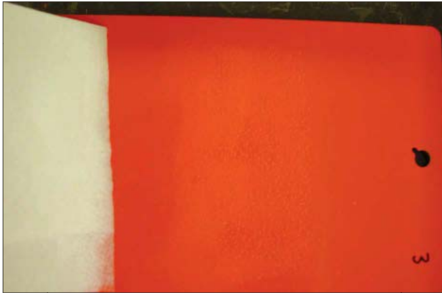
Fig. 1: The test panel with System #1 (specified system) showed discoloration and blisters after moisture exposure. Photos courtesy of KTA-Tator, Inc.
