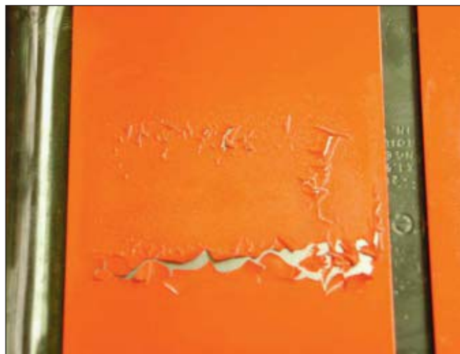
Fig. 3: The test panel for System #1 (specified system) exhibited cracking and delaminating coating.
