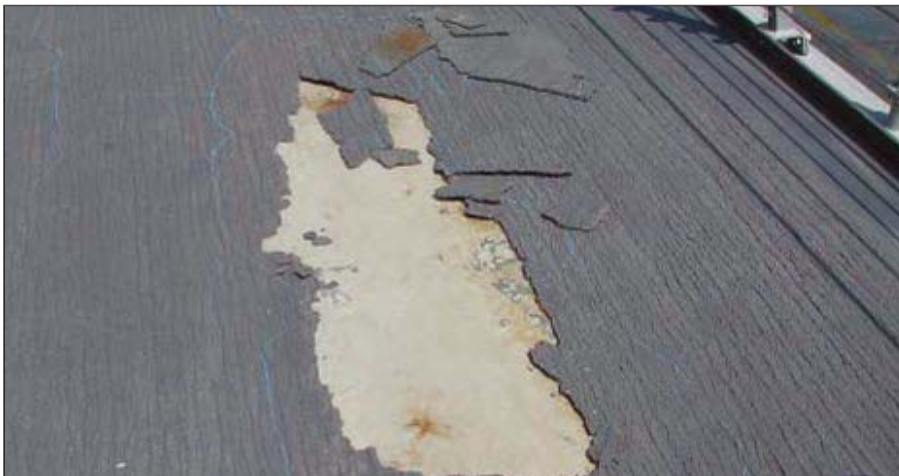
Fig. 1: Delamination failure case of slip-resistant coating film on the exposed deck of a marine vessel. Figs. 1-7 courtesy of the authors
