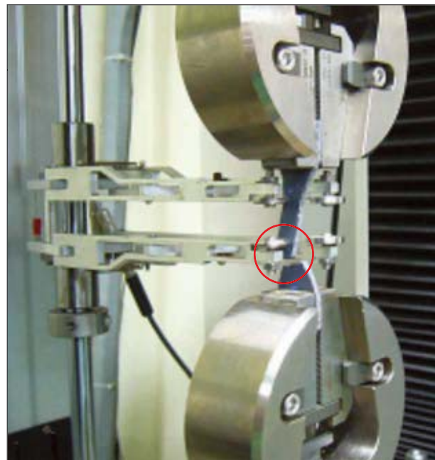
Fig. 5: Broken tensile specimen of high-build epoxy free film during installation
