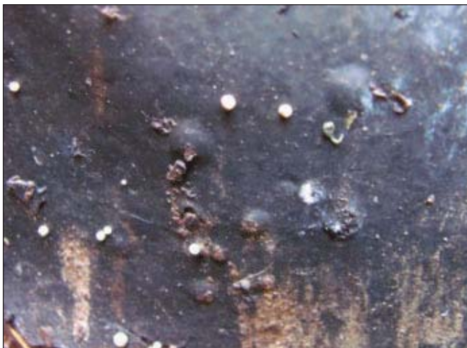
Fig. 4: An example of the white deposits (gypsum) found on some of the blister caps
