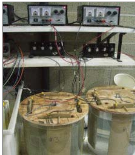
Cathodic disbondment testing in accordance with ASTM G8.
