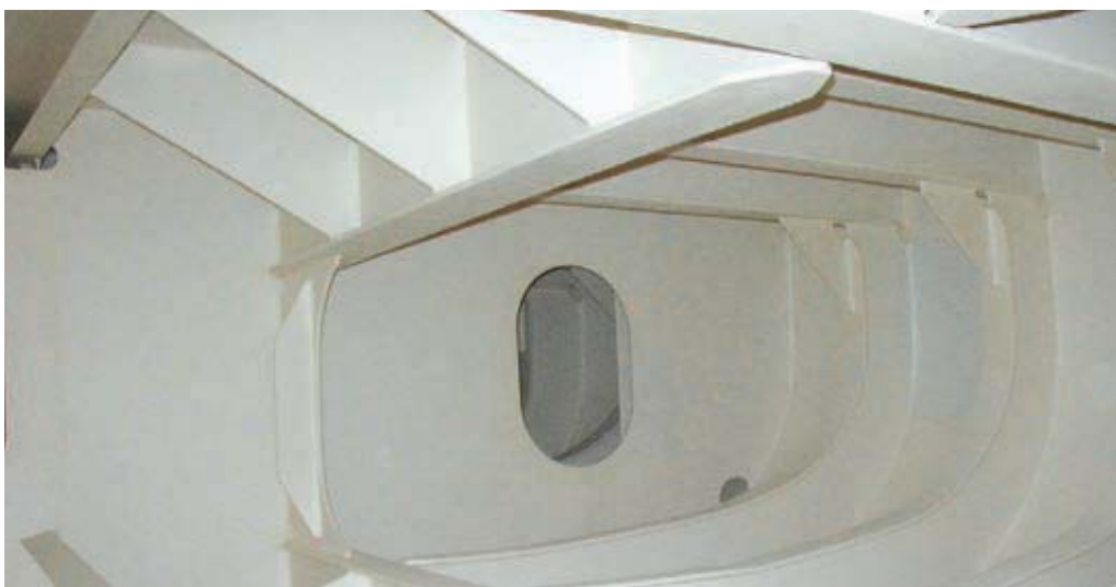
(Above): Ballast tank with lining in good condition. Courtesy of Exova (Facing page): Ship discharging ballast water. Courtesy of OceanSaver
