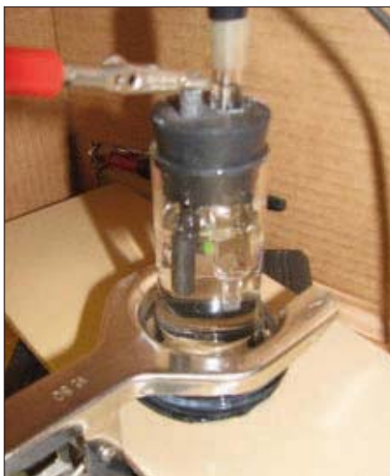
Testing coating impedance by electrochemical impedance spectroscopy (EIS). Photos courtesy of KTA-Tator, Inc.
