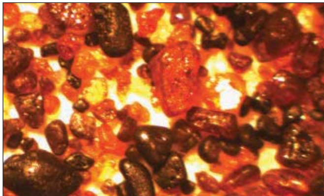
Extra fine staurolite abrasive under magnification
