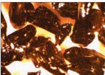
Fine iron silicate abrasive (copper slag) under magnification
