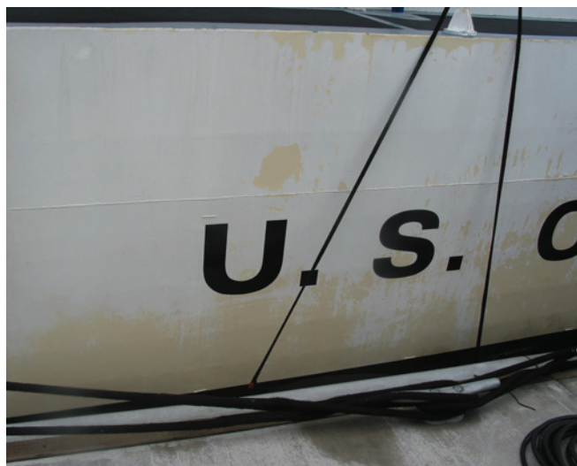
Fig. 3: The silicone alkyd beneath the black letters and markings did not delaminate or peel.
