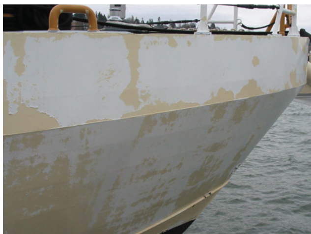
Fig. 1: Appearance of the starboard side where the alkyd silicone finish coat has cracked and peeled, exposing the underlying epoxy coat. All photos are courtesy of KTA-Tator, Inc.
