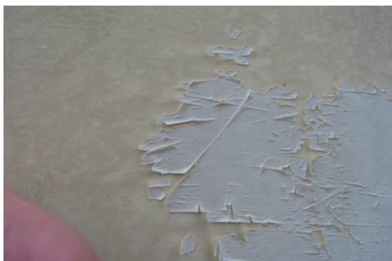
Fig. 2: The lighter color coating was all that remained of the exposed silicone acrylic finish coat on this freeboard section.
