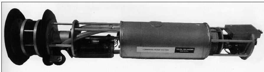
Fig. 3: Simplified photo of a centrifugal blast cleaner with two inflatable seals.
