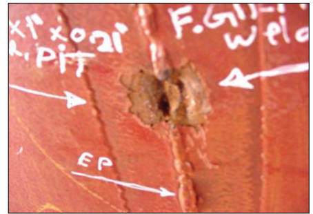
Fig. 9: Close-up of steel that was perforated in service due to a coating holiday.
