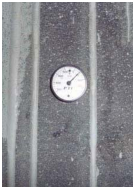
Fig. 1: Heavy coating runs on the bottom shell wall of the demineralized water tank. (The steel temperature was 48 F)
