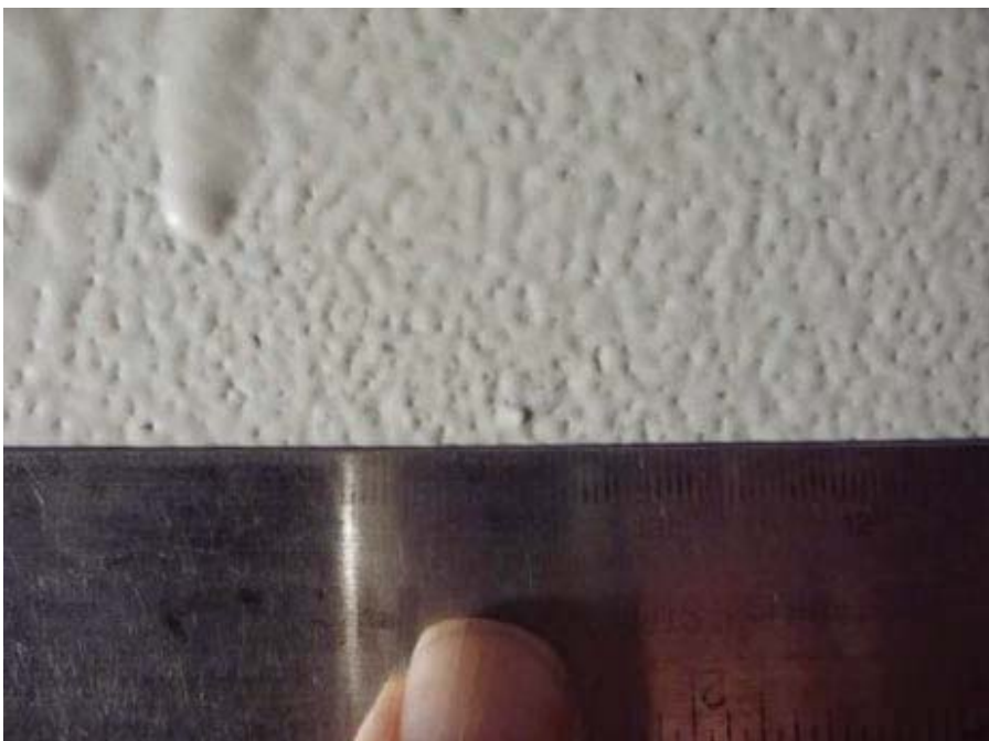
Fig. 5: Orange peel (and runs) on the face of the water overflow trough. The texture has features that may include pinholes. The DFT was 14–16 mils.
