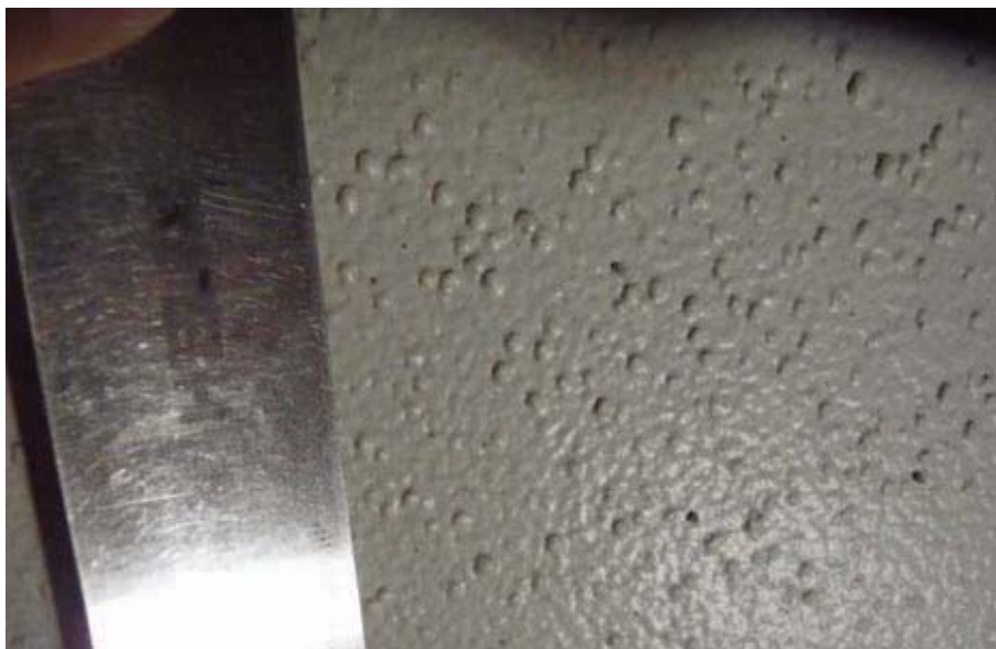
Fig. 6: A cluster of pimples on the surface of the coating. These may be droplets of coating that did not integrate into the film or bridged film over vapor filled voids. Several void holes are also present.
