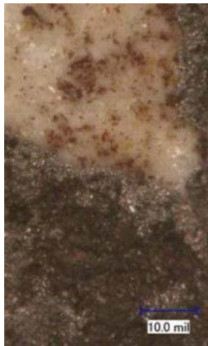
Fig. 7: The black scale rust discoloration on the back surface of Sample 1.
