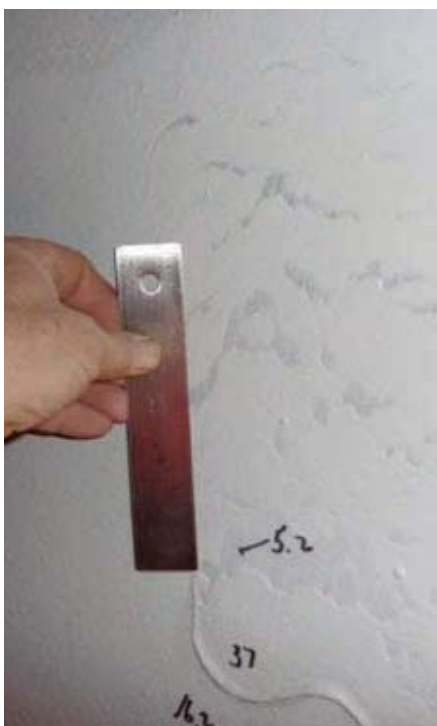
Fig. 4: The coating separated as it “slid” down the shell wall, leaving a thin layer behind (e.g., 5.2 mils).
