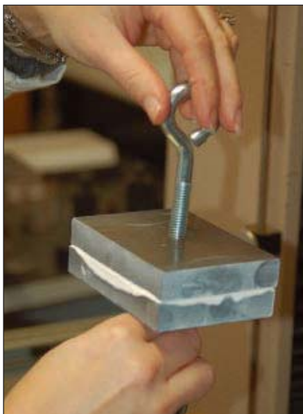
Fig. 4: Threading pulling rods to back sides of compression panels
