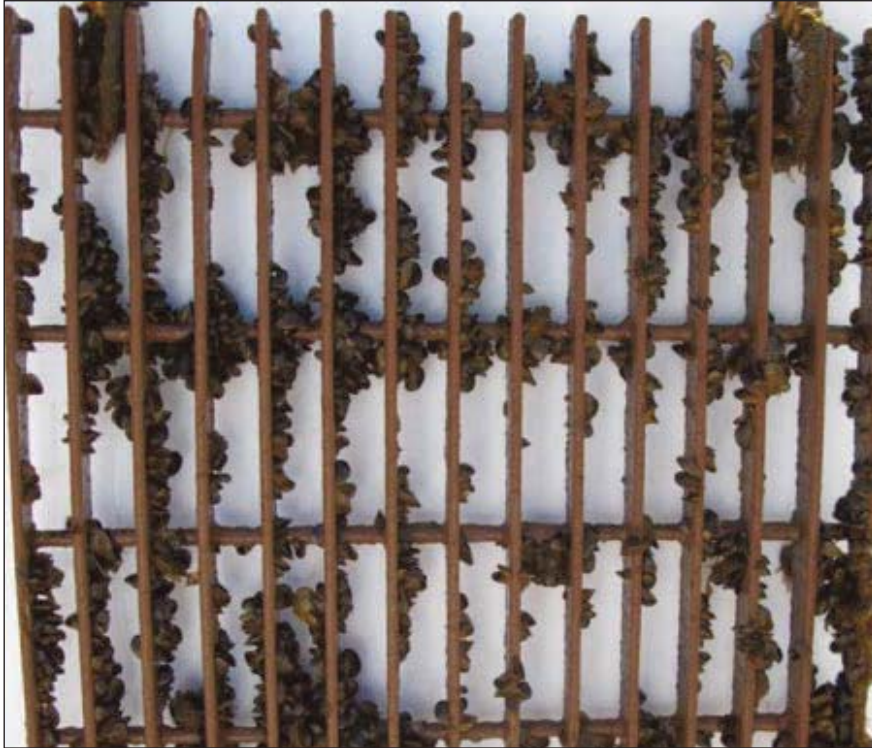
Fig. 8: Polyester filled with copper metal pigments.
