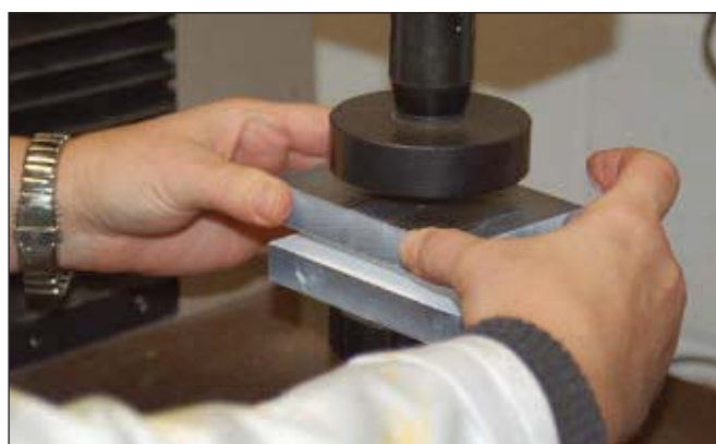
Fig. 2: Aligning mating surfaces for compression load
