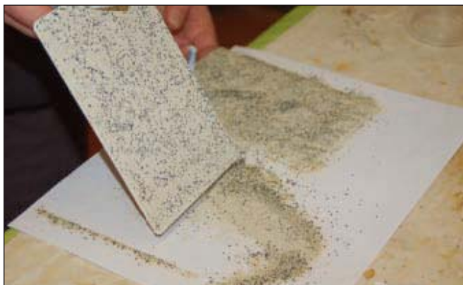
Fig. 1: Removal of abrasive/dust blend after one hour of dwell time.
