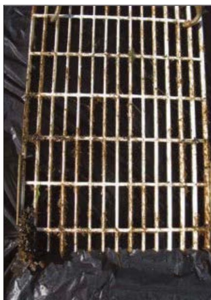
Fig. 6: Silicone foul-release coating #1 exposed for 2 years.
