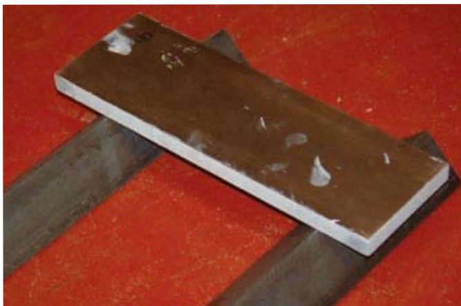
Fig. 6: Positioning of panel on apex of 1-inch angle iron (coated side down) for contact point test
