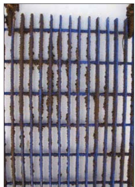
Fig. 7: Fluorinated silicone foul-release coating exposed for 2 years.
