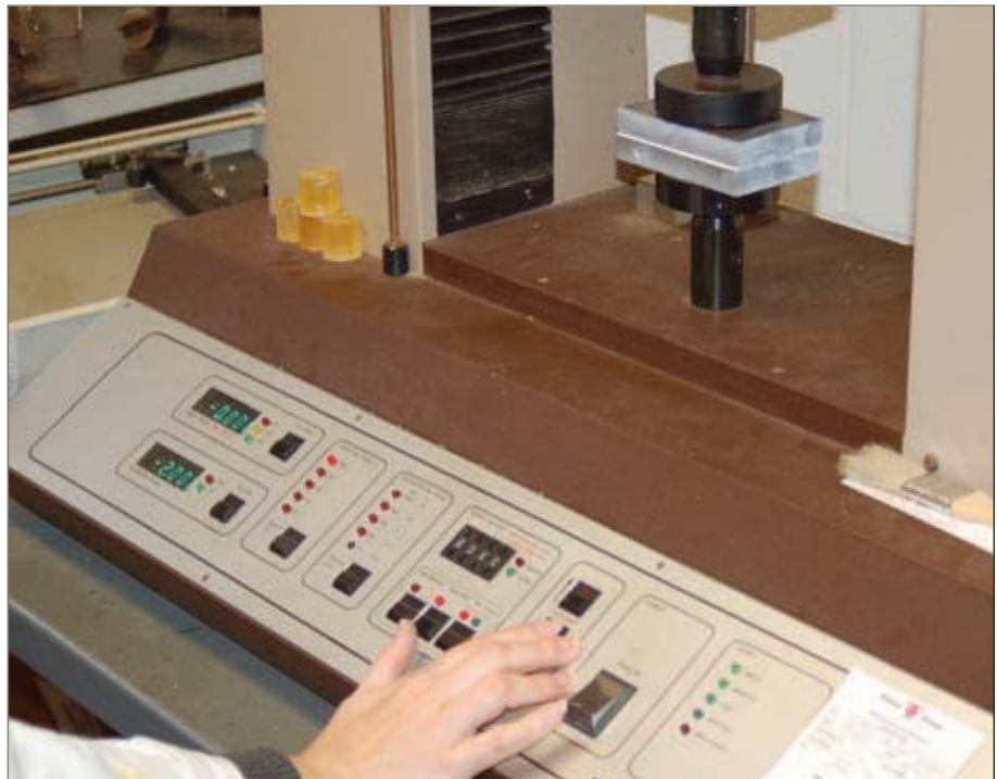
Fig. 3: Application of 260 lbs of force to mating surfaces
