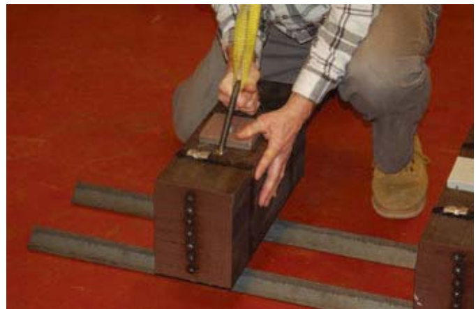
Fig. 7: Application and positioning of weight onto coated panel for contact point test
