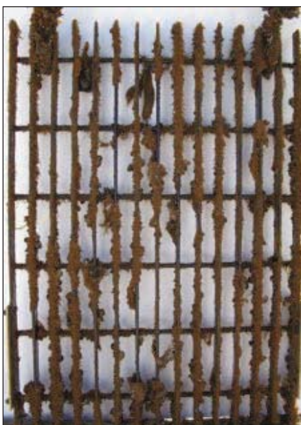
Fig. 5: Silicone foul-release coating #2 black color exposed for 1 year.
