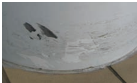
Fig. 16: Poor coating adhesion to ceramic enamel
