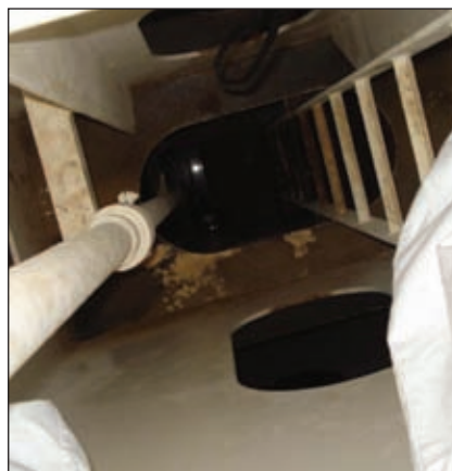
Fig. 4: Interior of a coated fore peak tank with ladders and climbing irons
