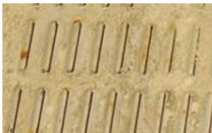
Fig. 12: Sample piece of louver with rust spots and rust stain
