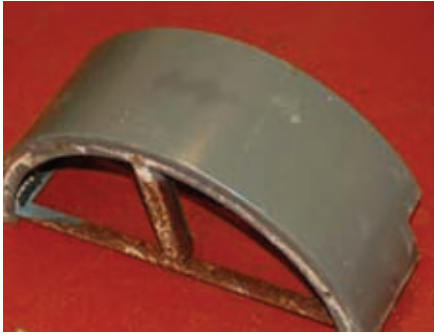
Fig. 11: Corrosion at base of steel column began in its hollow interior
