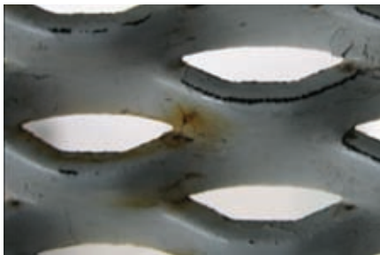
Fig. 4: Magnified view of rusty grating/screen on some porcelain-enameled panels
