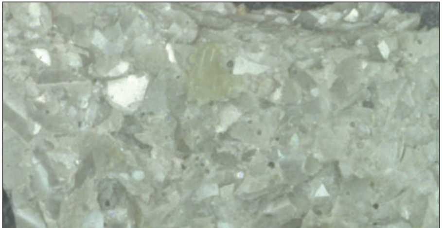
Cohesive split in the gray topcoat after trying to remove discoloration on the top surface. Photos are not to scale. All photos are courtesy of KTA-Tator, Inc.
