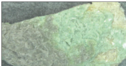
Cohesive split in the two base coats and the topcoat after trying to pry the coats apart.
