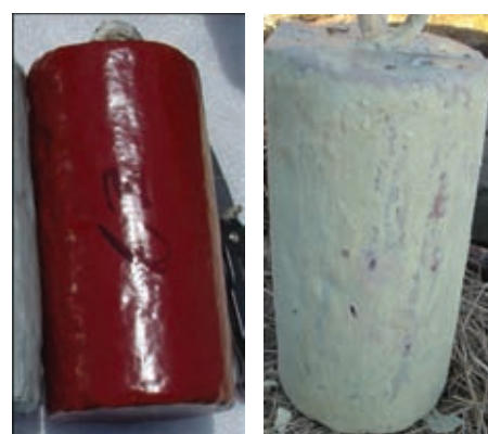
Fig. 13: South TX: 55% volume solids polyamide epoxy applied at 17 mils DFT to concrete cylinder panel before 12-month exposure (left) and following 12-month exposure (right).
