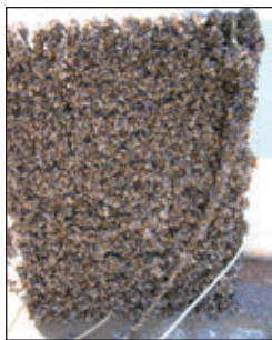
Fig. 4: Uncoated steel floor grate in dynamic conditions at 7 months of exposure.
