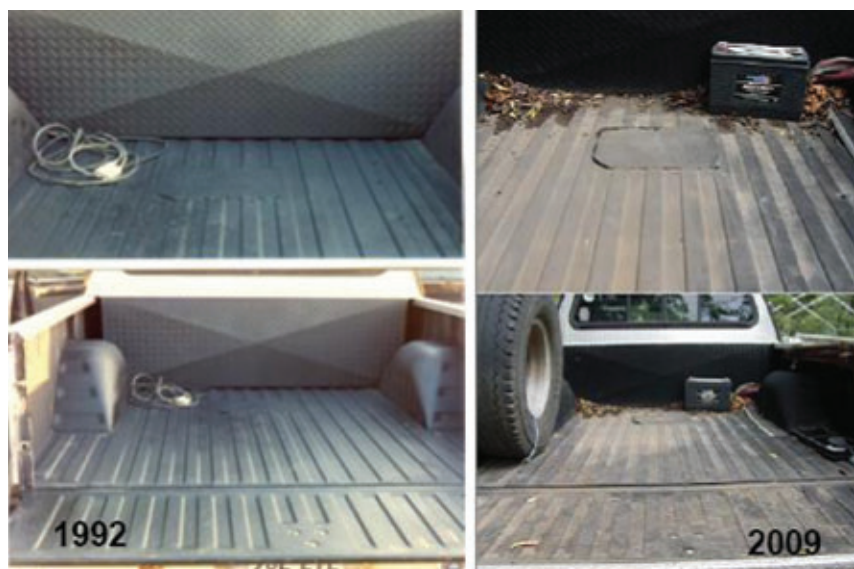
Fig. 2: Bedliner—before and after
