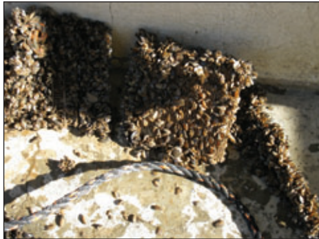
Fig. 5: 90/10 Copper/nickel alloy in static conditions after 4 months of exposure.
