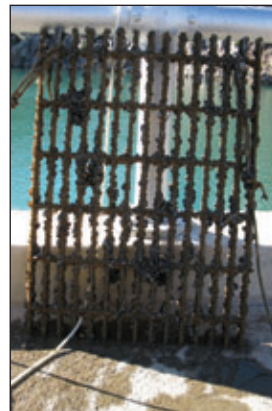
Fig. 6: 100% zinc metallized grate at 7 months exposure.
