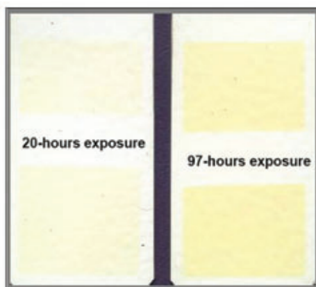
Fig. 3: Aliphatic modified aromatic polyurea QUV weatherometer exposure, UVB-313 Bulbs
