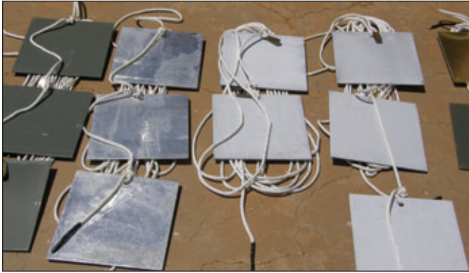
Fig. 2: Coated square foot steel plates used for static testing. From left to right: zinc-rich epoxy, galvanized, 85-15 zinc-aluminum metalized, 100% zinc metalized, and copper metal.
