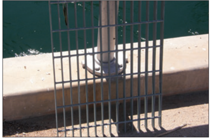
Fig. 3: Coated steel floor grate used for dynamic testing.
