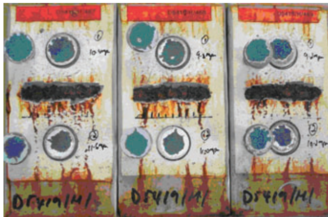
Fig. 8: Three panels tested per ISO 20340 for scribe cutting. The left and middle panels passed; the panel on the right failed; hence, the problem with assigning arbitrary pass-fail values.
