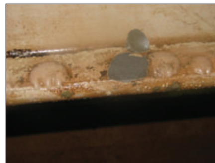
Fig. 2: Blister with no oxygen permeation (without rust)
