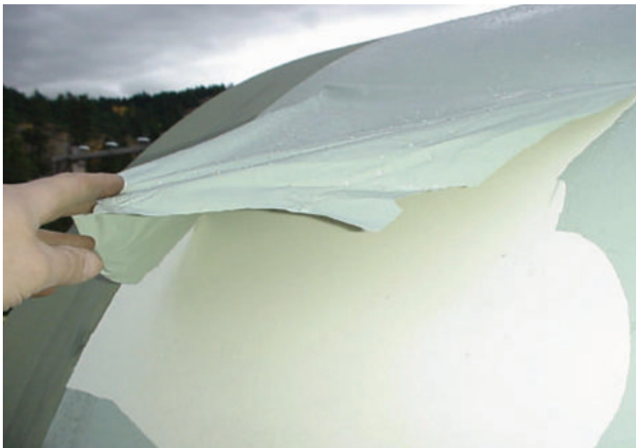
Fig 5: Example of a polyurethane finish coat applied beyond the recoat window of an epoxy mid-coat. Intercoat adhesion between the polyurethane and epoxy mid-coat is best determined by wet adhesion testing as opposed to dry adhesion testing.
