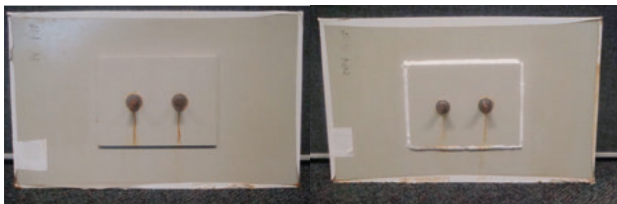
Fig. 3: Cycle 6 results on stud-welded panels
