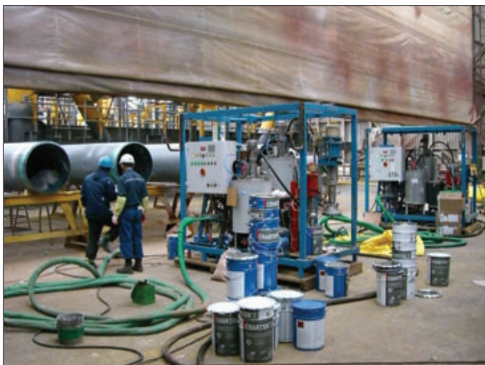
Fig. 4: Units for plural-component application of intumescent. Photo courtesy of WIWA GmbH
