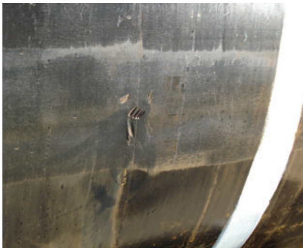
Fig. 13: Coating damaged from nails on wedge support
