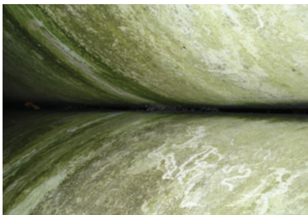
Fig. 6 (Top): 28-ton concrete coated pipes on the pipe stop
