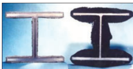
Fig 1: Intumescent coating applied to steel beam (left) and after the coating has been exposed to heat/fire and has expanded (right). Photo courtesy of International Paint
