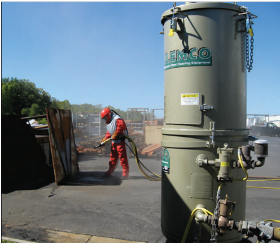
Fig. 1: Effective and safe abrasive blasting requires the correct equipment and setup as well as a properly trained operator. All figures and tables are courtesy of Clemco Industries.
