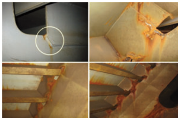
Fig. 8: Cracks related to excessively hard paint with inadequate elasticity.
