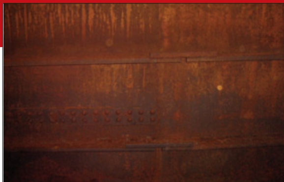
(Facing page): DPST Ataulfo Alves. In 2002, the bottom plating of all cargo tanks were UHP hydro-blasted and painted with 2 coats (150 \mu\text{m} each) of WST epoxy paint, in white color. Still today the coating looks brand new. All photos courtesy of the author. Fig. 1 (above): Ballast tank of an old ship, not coated. Fig. 2 (right): Ballast tank coated with CTE paint (18 years). Rare example of tank well coated and well maintained.
