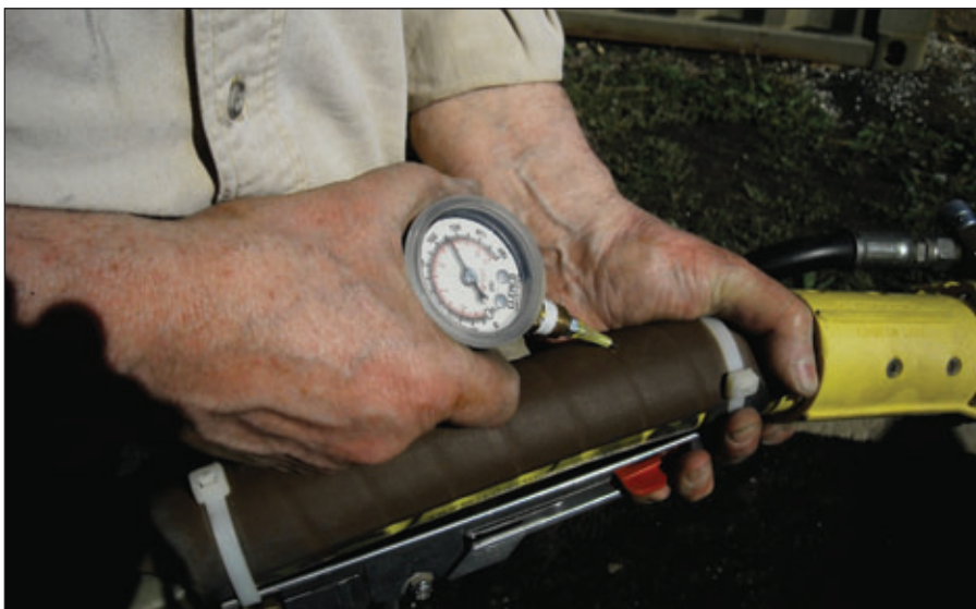
Fig. 2: Needle pressure gauge used to check pressure at the nozzle.
