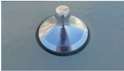
Fig. 4a: Testing surface tensile strength properties using 50-mm-diameter dollied in accordance with ASTM D 7234
