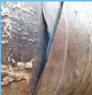
Fig. 1: Lack of adherence of HSS on PE (top) and steel (below) on 18-inch Gabon. All photos courtesy of the authors.
