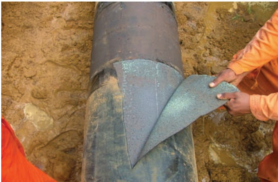
Fig. 3: Disbonding of 3LPE at 35^{\circ}\text{C} [ 95^{\circ}\text{F} ] 18-inch Gabon)
