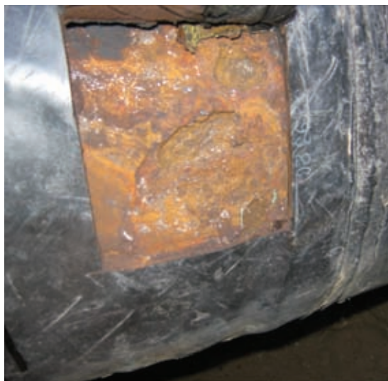
Fig. 2: Heavy corrosion under disbonded HSS (16-inch Syria)
