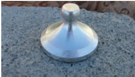
Fig. 4b: Testing surface tensile strength properties of Concrete Control Panel A (SSPC-SP 13/NACE No. 6, ICRI-CSP5 prepared concrete panel) using 50-mm-diameter dollied in accordance with ASTM D 7234.
