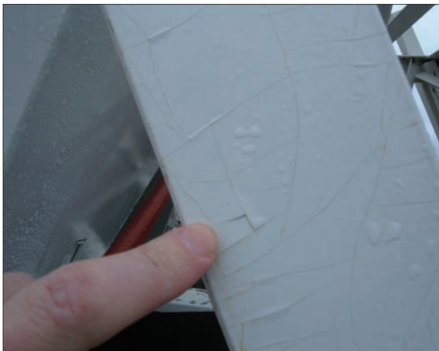
Fig 2: More cracking in the coating system was observed in areas with increased coating thickness.
