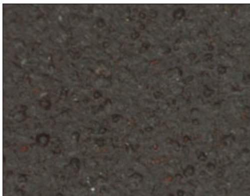
Fig 3: Magnified view of back side of a coating sample showing a black color with spots of red (primer).
