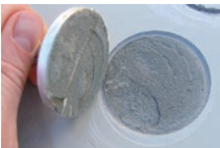
Fig. 7c: Surface tensile strength failure planes were determined by observing the bottom of the 50-mm dollies.
