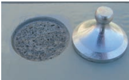
Fig. 4c: Evaluating surface tensile strength properties of Concrete Control Panel B.
