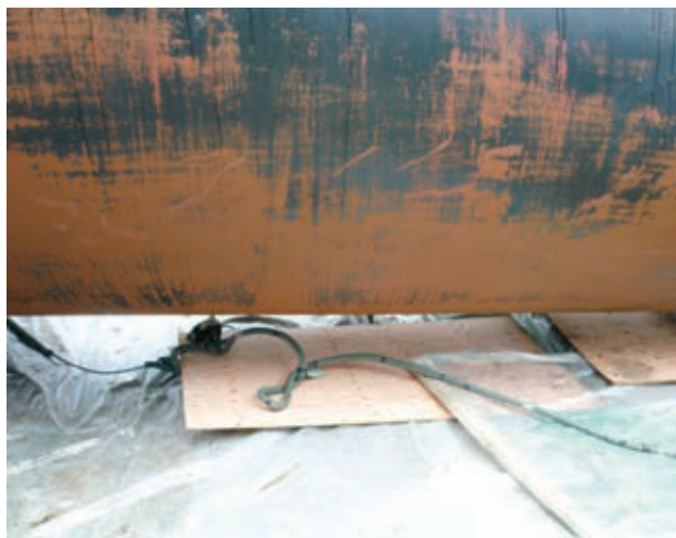
Fig. 9: View of lead-based alkyd primer after pressure washing
