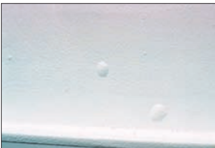
Fig. 6: The blisters probably occurred because moisture was on the surface before coating application.
