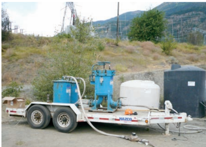
Fig. 7: Truck-mounted filtration units for the supernate from the holding tanks
