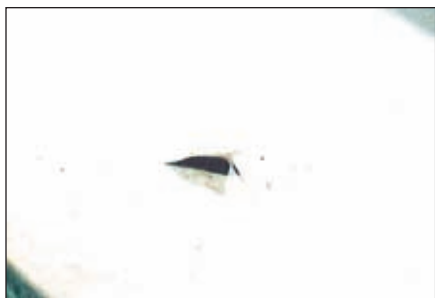
Fig. 4: ASTM D6677 adhesion tests showed poor adhesion values (0).
