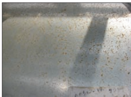
Fig. 2: Steel supplied by the North Central fabricator developed pinpoint rusting on the primer. The dry film thickness ranged from 2.0 to 4.9 mils.
