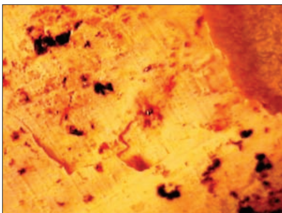
Fig. 4: Sample KTA-3, viewed at 40X magnification, shows the appearance of pinpoint rusting of primer modified with curing accelerator.
