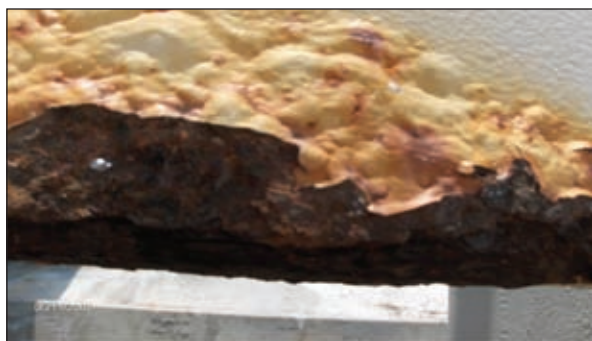
Spot of luminal corrosion on the lower ring of a railing
