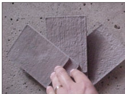
Fig. 1: ICRI No. 03732 Visual CSP Templates against abrasive blasted concrete surface
