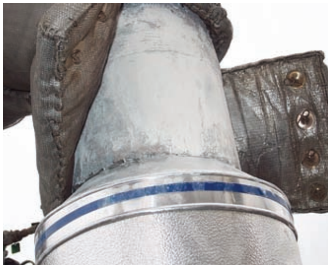
Fig. 2: Insulation blanket is folded back to show failed silicone aluminum over relatively intact aged inorganic zinc.
