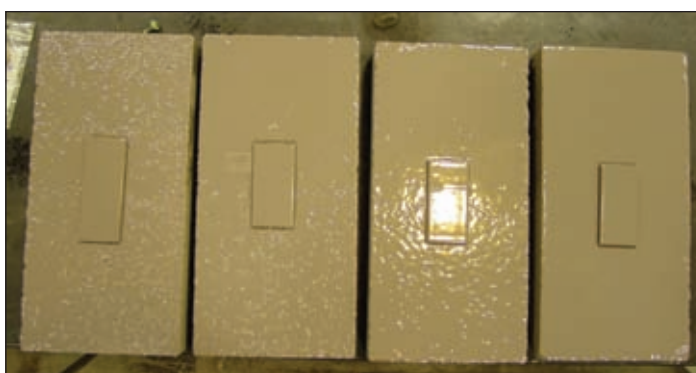
Fig. 4: (L to R) Coated concrete test samples, one coat to four coats
