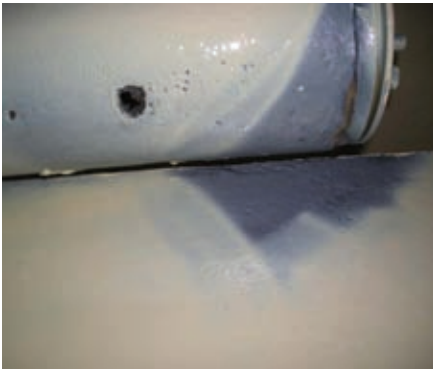
Fig. 6: Excessive millage created an unusual sag on the bulkhead and had to be sanded off
