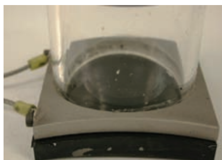
Fig. 9: Slipping experiment (pulling panel is the bare steel panel attached to the coating)
