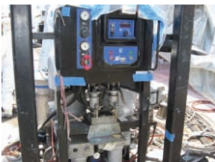
Fig. 3: The report recommends dedicating a set of spray lines of plural-component equipment to one coating system
