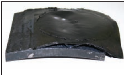
Slippage after 3 days with 10 kg (22 lb) load
