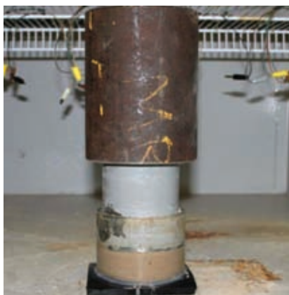
Fig. 4: Piston arrangement to simulate soil stress
