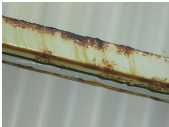
Fig. 4: Coating breakdown at an edge
