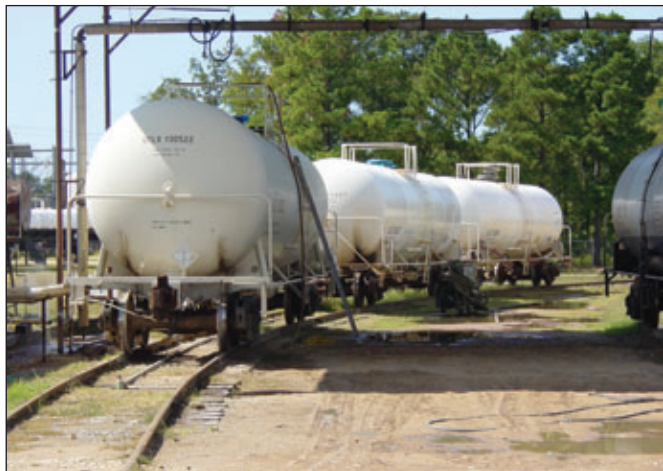
Tank car that transports hydrochloric acid as it awaits cleanout and inspection. Photo by Danny Lee. Courtesy of Blair Rubber Company
