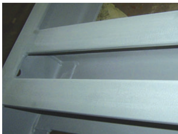
Fig. 5: Difficult-to-access regions are difficult to paint, and DFT is difficult to measure on them.
