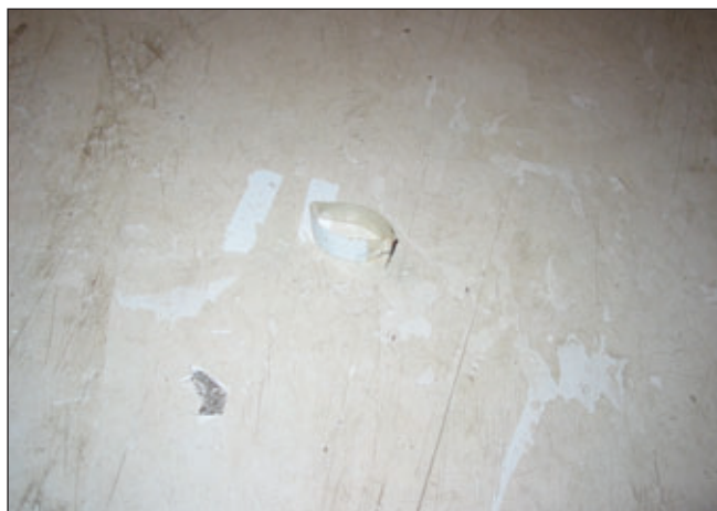
Fig 2: ASTM Tape Test revealed poor coating adhesion
