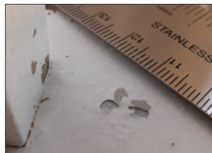
Fig 4: (Case 2) Small blister caps were lifted from the coating film with a knife tip, exposing the aluminum substrate. These were located near, and appeared associated with, filiform strands. Not to scale.
