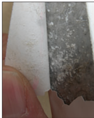
Fig 1: (Case 1) Surface soiling shows the area of a split film exposed to weather. the white corrosion products include aluminum hydroxides and oxides that are somewhat dry (not fully hydrated).
