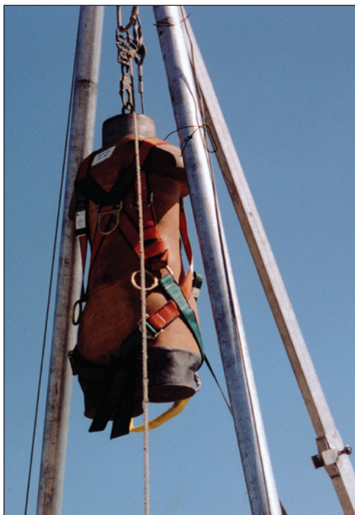
ANSI test torso rigged for demonstration drop in fall protection training. Courtesy of MSA
