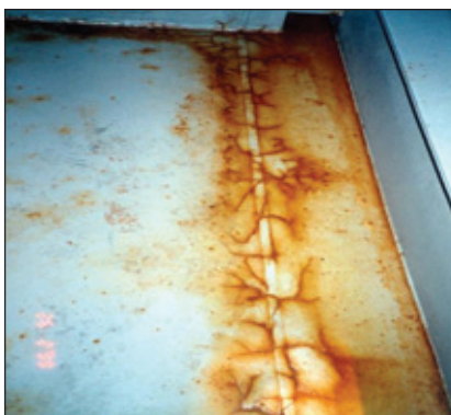
Fig. 1: Typical example of cracking at the weld
