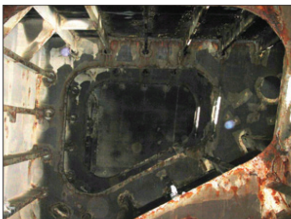
Fig. 2: Typical condition of tar epoxy system in topside WB tank after 7–8 years, using present methods and coatings
