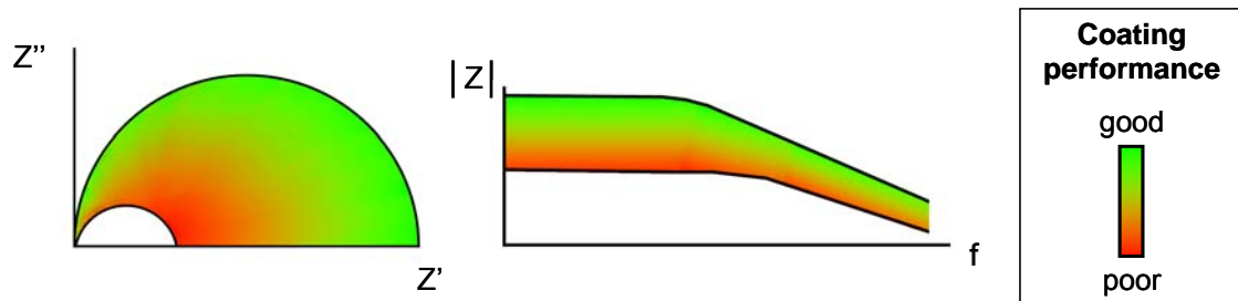
Figure 1 EIS spectra for different levels of coating performance, left Nyquist plot and right a Bode plot.
