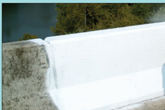
Portion of barrier coated for atmospheric testing Photos courtesy of the authors
